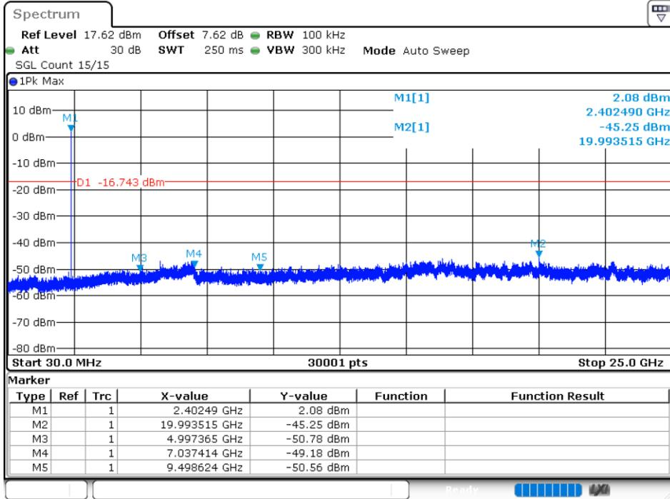
Tx. Spurious NVNT GFSK 2440MHz Ant1 Ref
