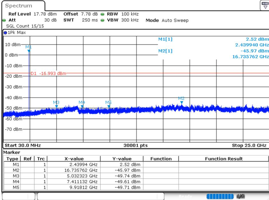
Tx. Spurious NVNT GFSK 2480MHz Ant1 Ref
