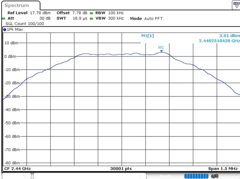
Tx. Spurious NVNT GFSK 2440MHz Ant1 Emission
