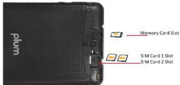
3. Push in the sim card slot and power on the tablet.
