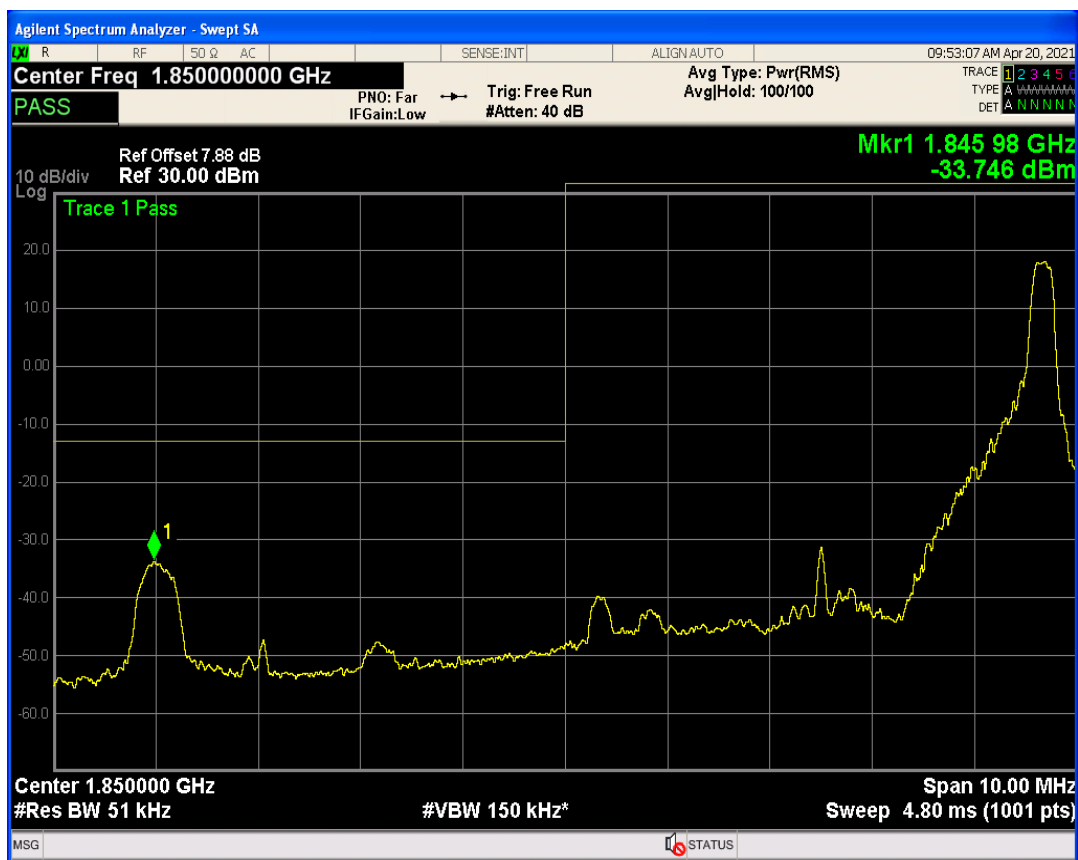
Band2 QAM16 BW=5MHz Channel=18625 RB Size=25 Position=#0
