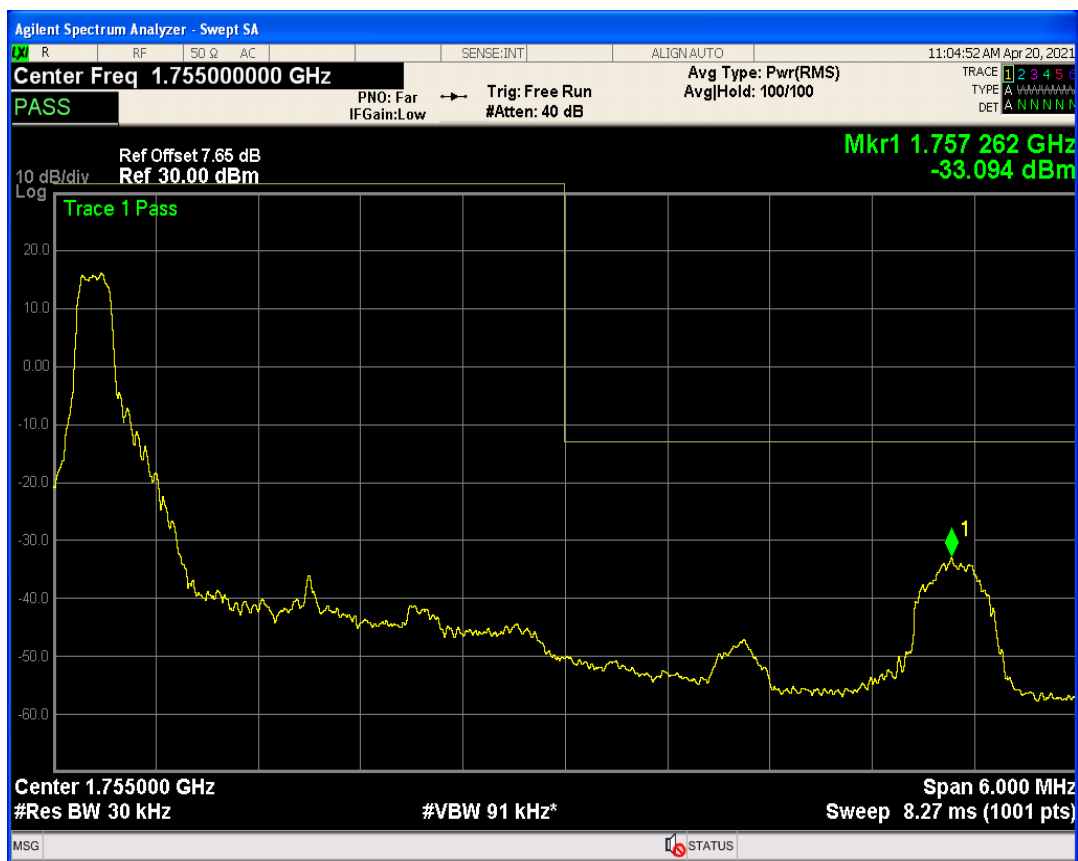
Band4 QAM16 BW=3MHz Channel=20385 RB Size=1 Position=#Max
