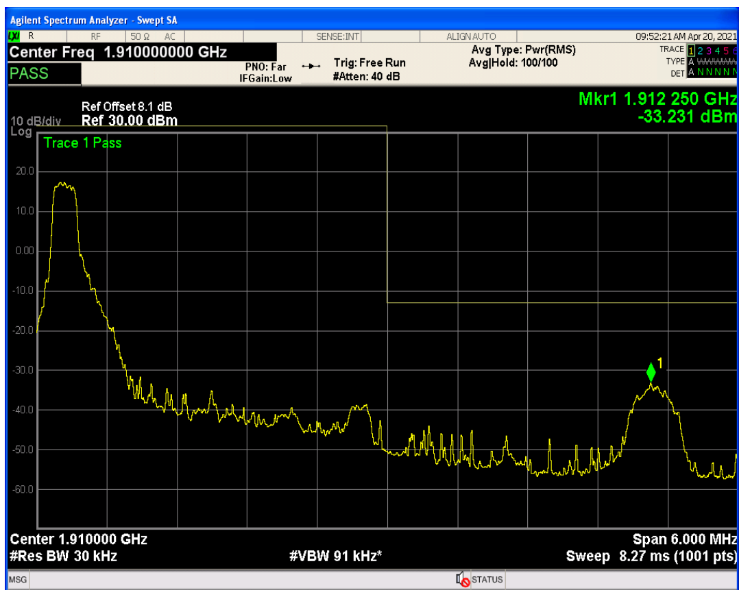
Band2 QPSK BW=3MHz Channel=19185 RB Size=15 Position=#0
