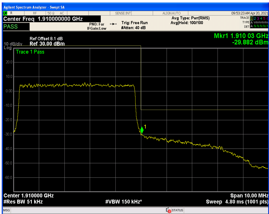
Band2 QAM16 BW=5MHz Channel=19175 RB Size=1 Position=#Max
