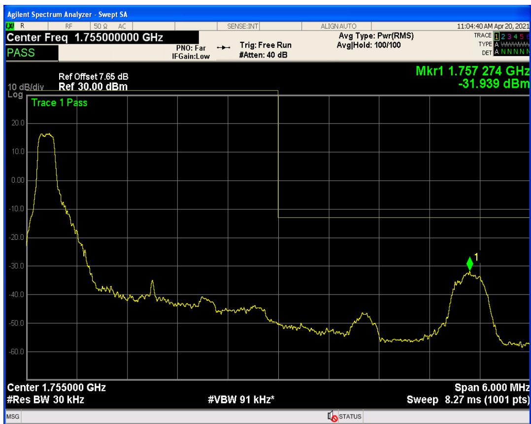
Band4 QAM16 BW=3MHz Channel=19965 RB Size=15 Position=#0
