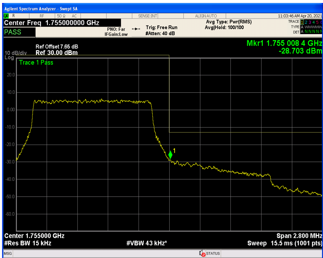
Band4 QAM16 BW=1.4MHz Channel=20393 RB Size=1 Position=#0
