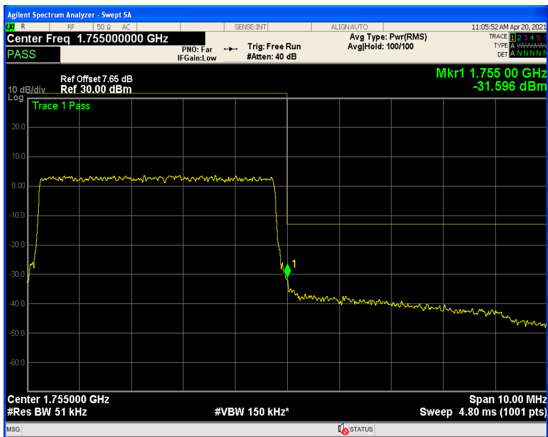
Band4 QPSK BW=10MHz Channel=20000 RB Size=1 Position=#Max
