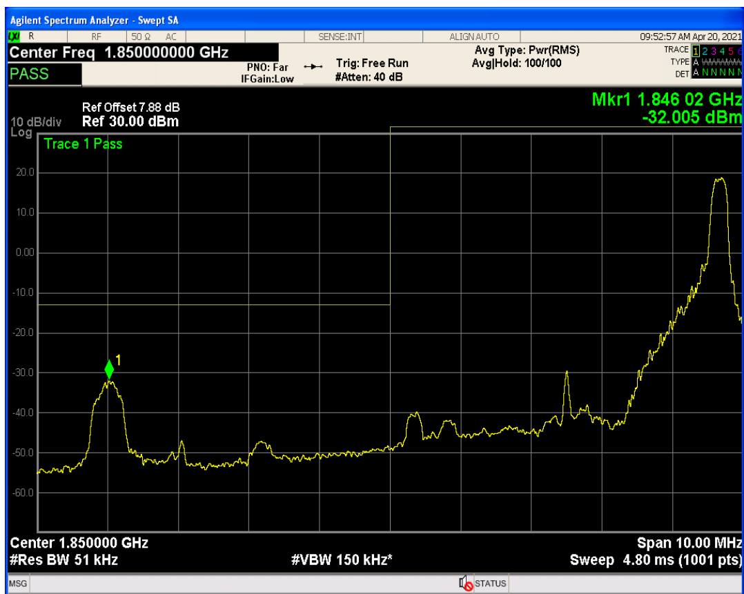
Band2 QAM16 BW=5MHz Channel=18625 RB Size=1 Position=#0
