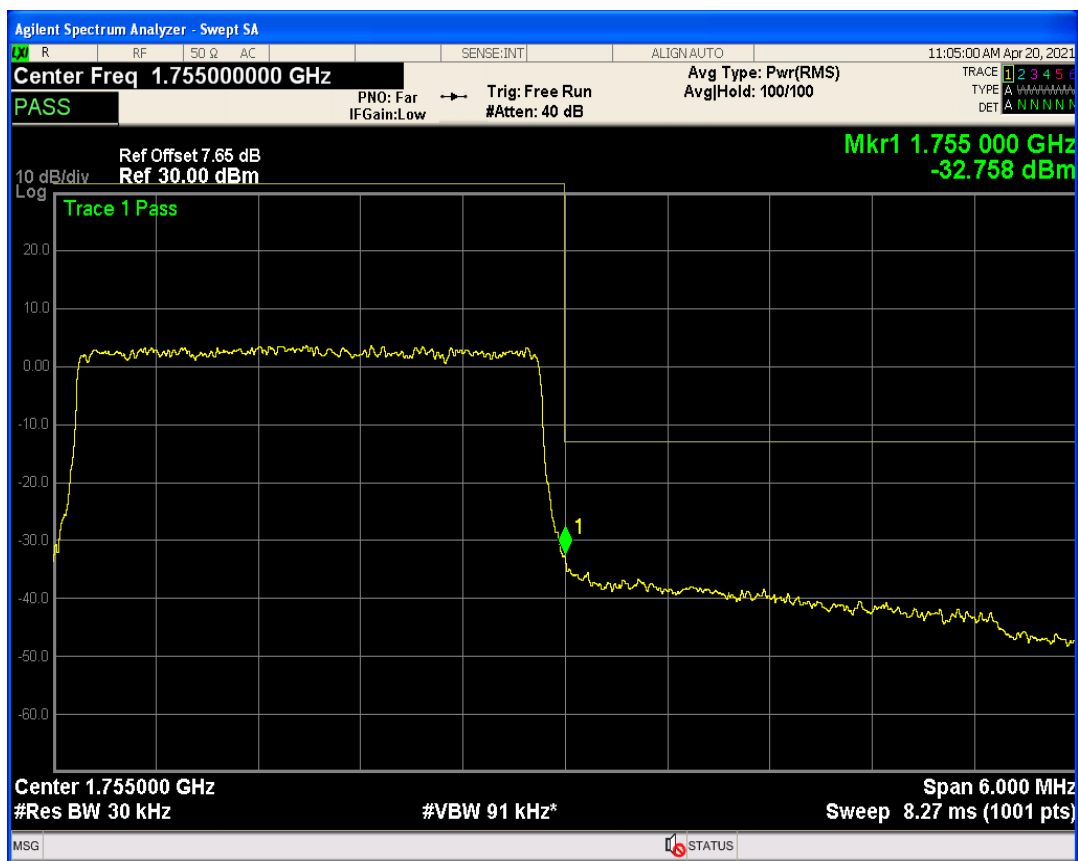
Band4 QPSK BW=5MHz Channel=19975 RB Size=1 Position=#0
