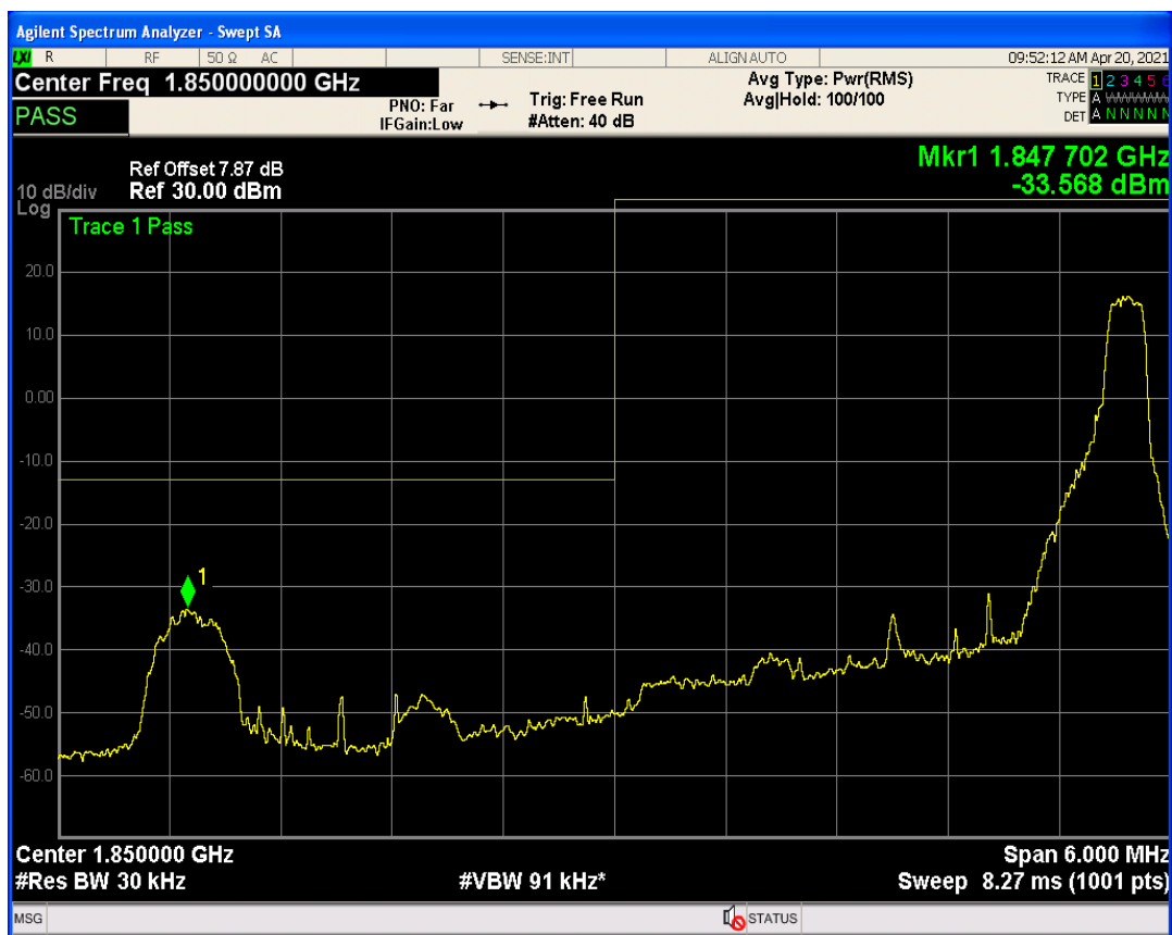
Band2 QAM16 BW=3MHz Channel=18615 RB Size=15 Position=#0
