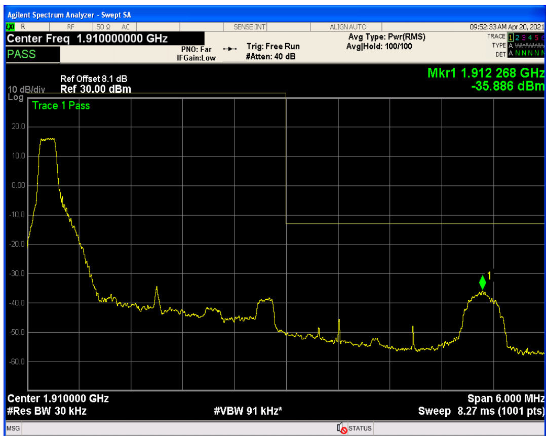
Band2 QAM16 BW=3MHz Channel=19185 RB Size=1 Position=#Max
