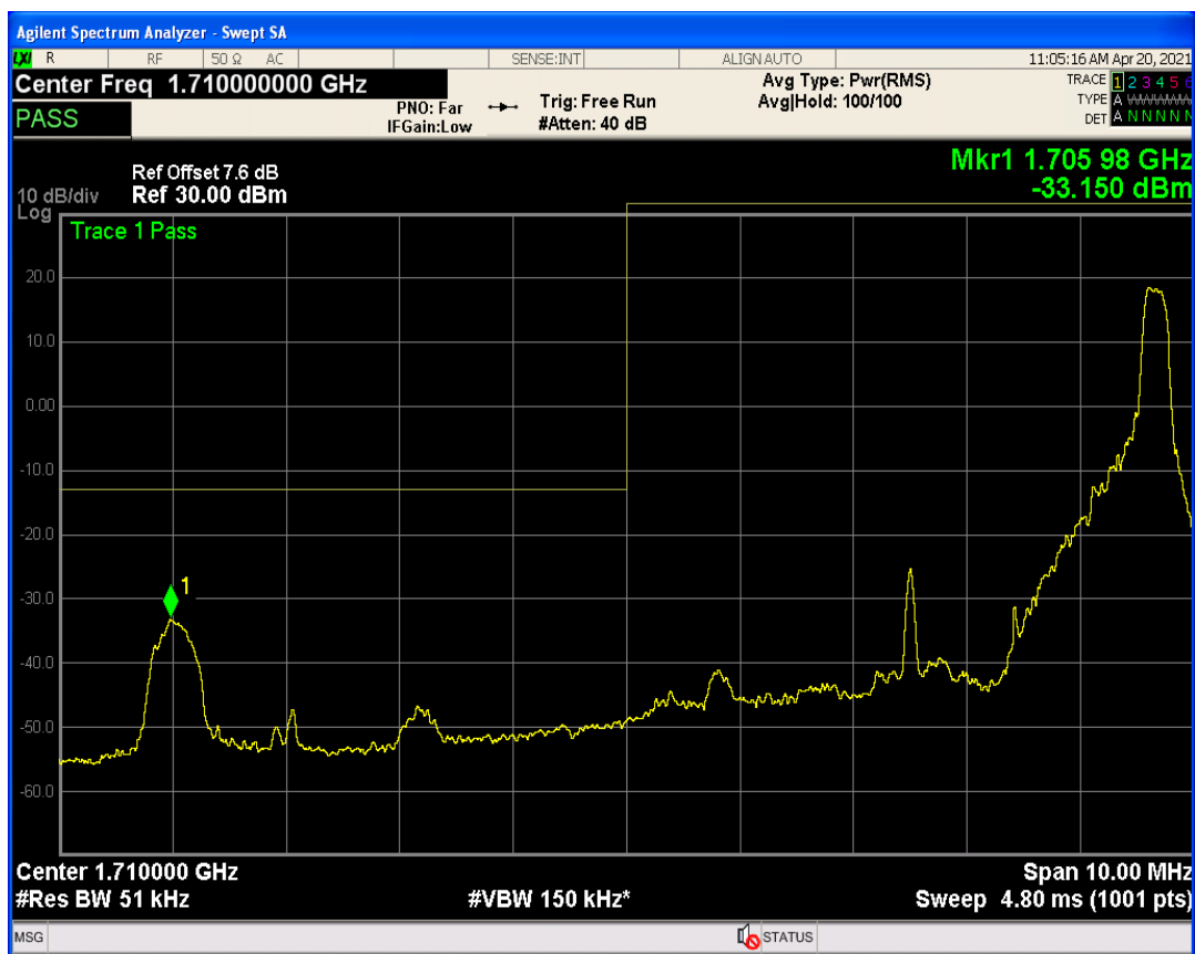
Band4 QPSK BW=5MHz Channel=19975 RB Size=25 Position=#0
