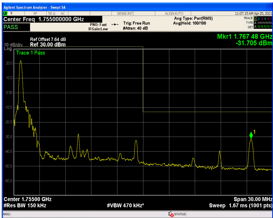
Band4 QPSK BW=15MHz Channel=20325 RB Size=75 Position=#0
