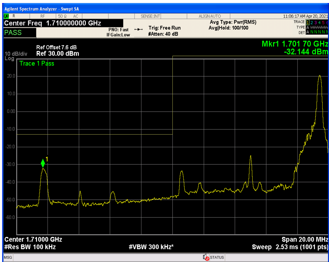
Band4 QPSK BW=10MHz Channel=20350 RB Size=1 Position=#0
