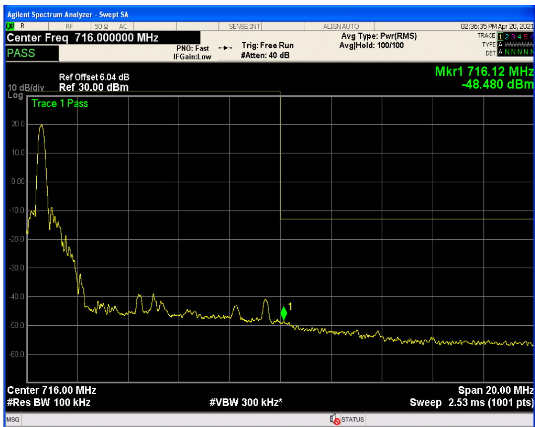
Band17 QPSK BW=10MHz Channel=23800 RB Size=50 Position=#0
