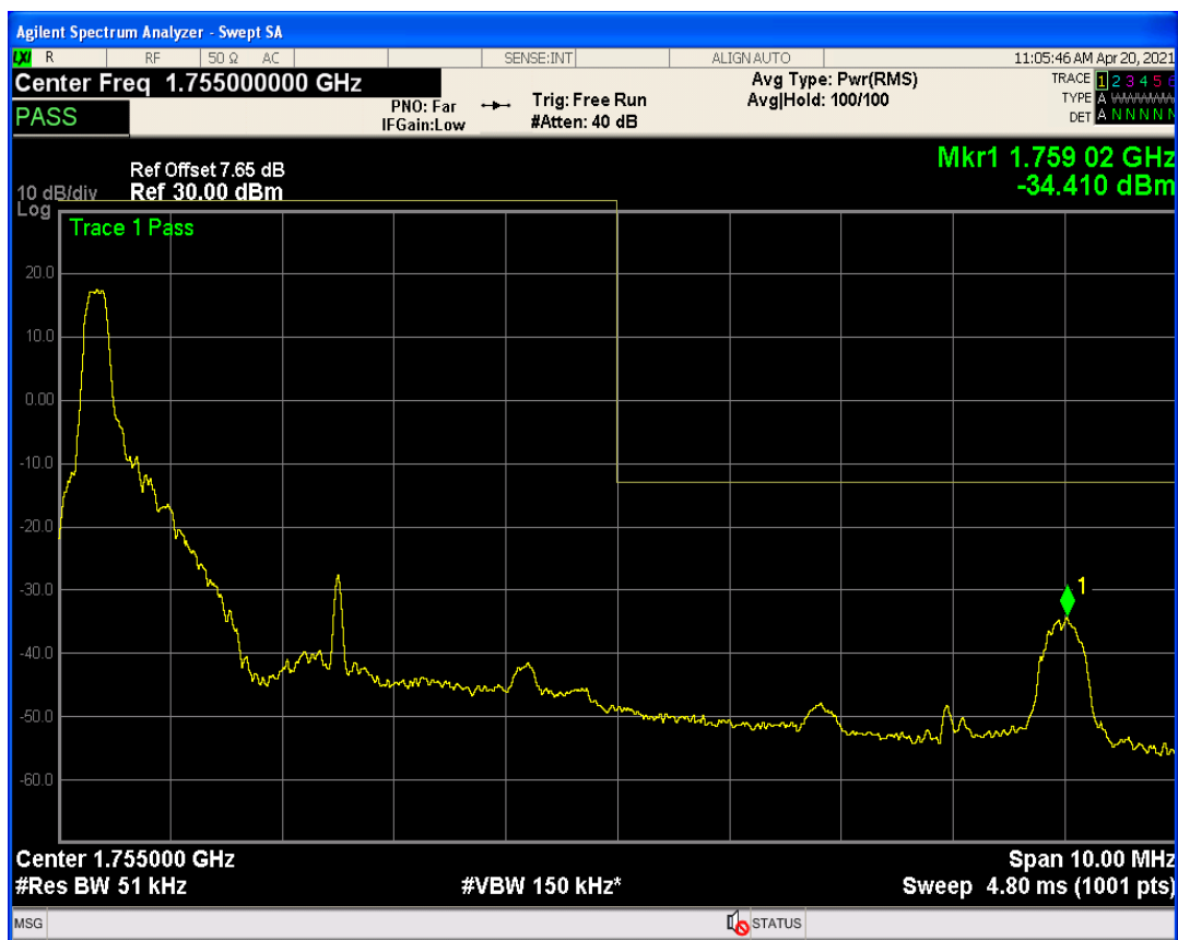
Band4 QAM16 BW=5MHz Channel=20375 RB Size=25 Position=#0
