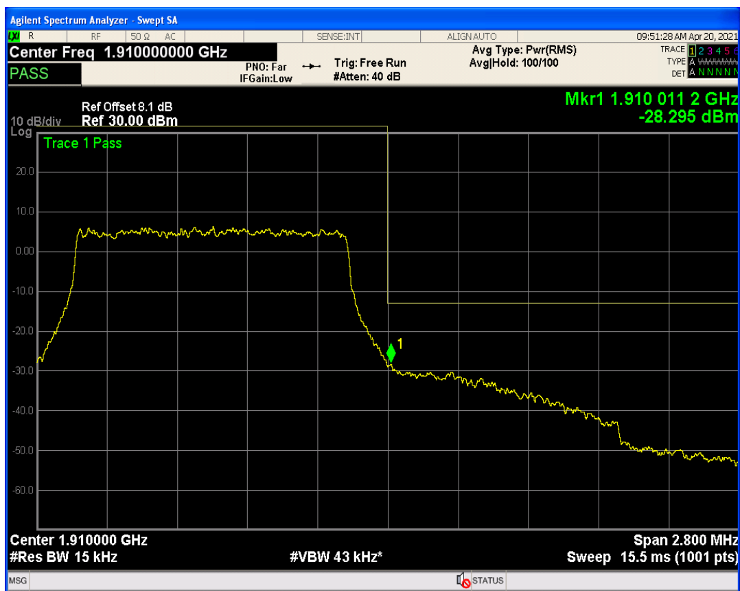
Band2 QAM16 BW=1.4MHz Channel=19193 RB Size=1 Position=#0
