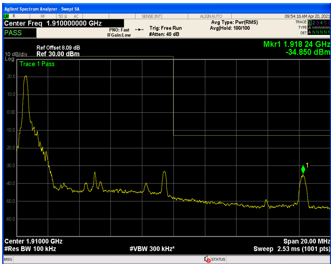
Band2 QAM16 BW=10MHz Channel=19150 RB Size=1 Position=#Max
