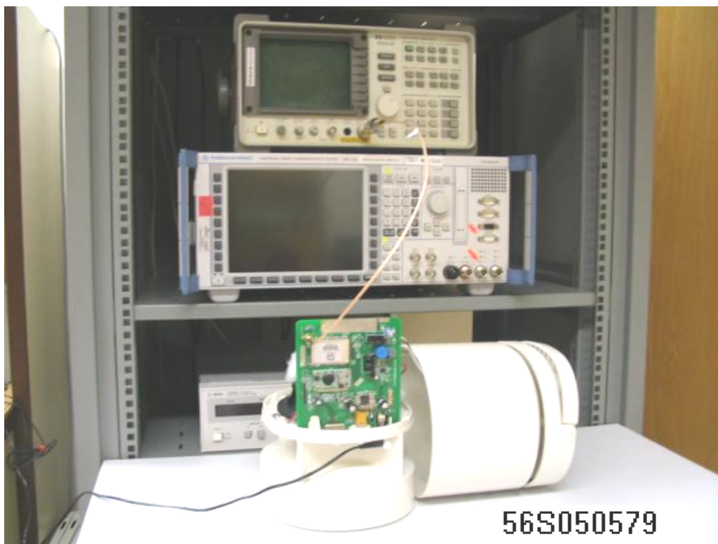
Number of Hopping Frequencies Measurement Test Setup
