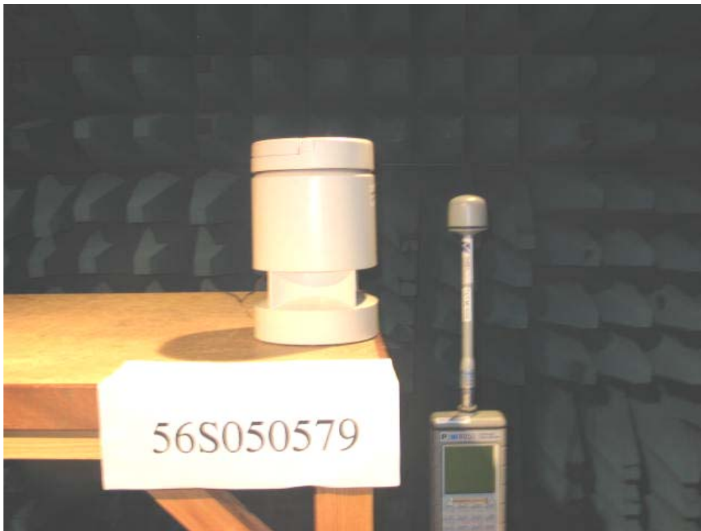
Maximum Permissible Exposure Measurement Test Setup
