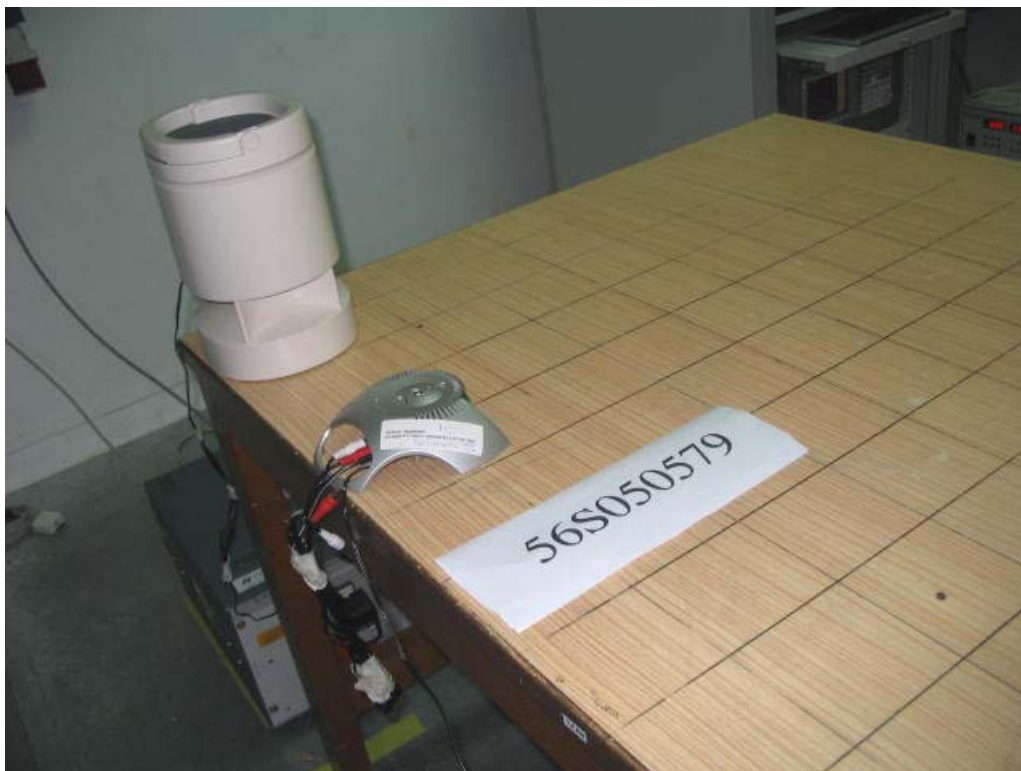
Conducted Emissions Setup (Rear View)
