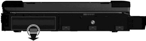
5. With the ribbon strip facing outward, insert the new battery pack all the way into the compartment.
