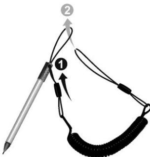
2. Insert the other loop end to the hook on the computer (as indicated by **1** below). Then, insert the stylus end through the loop (as indicated by **2** below) and pull it tight.
