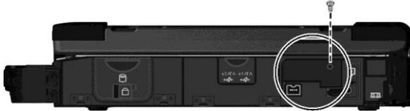
4. Insert the SIM card into the slot. Make sure the beveled corner on the SIM card is facing towards the slot and that the golden contact area on the card is facing downwards.
