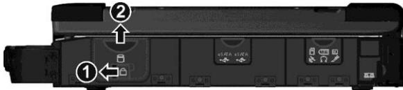
3. Pull the strip and slide the hard disk drive out of the slot.
