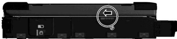
3. Press the eject button and the DVD tray will slide out partially. Gently pull on it until it is fully extended.
