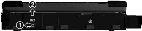
4. Pull the ribbon strip and slide the battery pack out of the compartment.
