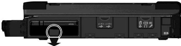
4. With the strip facing outward, insert the new hard disk drive all the way into the slot.
