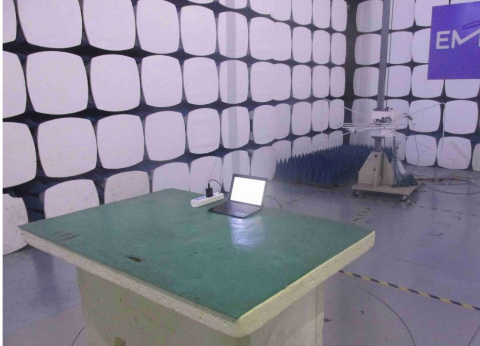
Photograph 2: Set-up for Spurious Emissions for 1 - 18GHz
