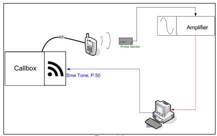
Figure 4-2 **T-Coil Test Setup**
