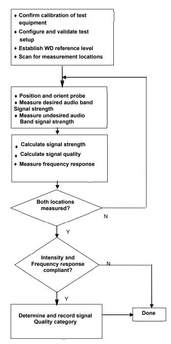
Figure 4-14 C63.19 T-Coil Signal Test Process
