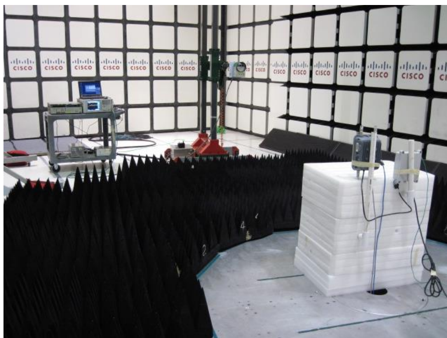
Radiated Test Setup 18–40GHz
