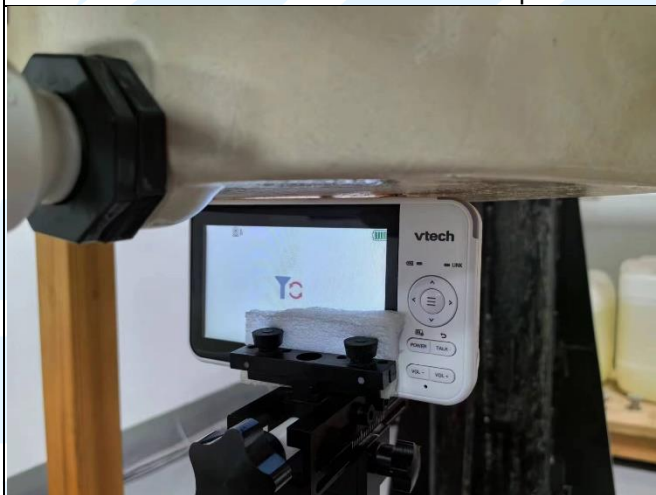
Top Side of EUT with 0 cm Gap
