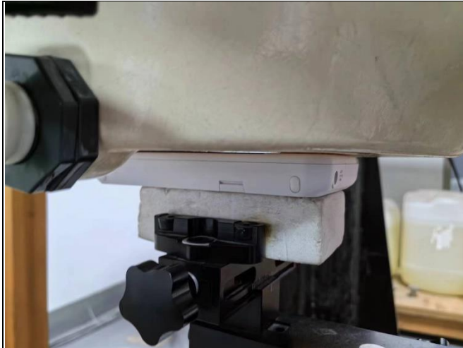
Front Face of EUT with 0 cm Gap
