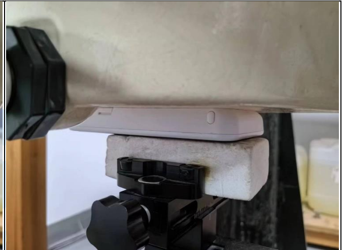
Rear Face of EUT with 0 cm Gap
