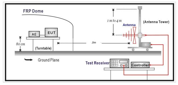
Above 1GHz Test Setup:
