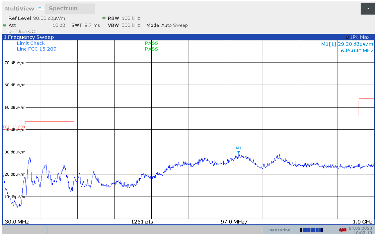
Radiated Emissions, 30 -1000 MHz, 2437 MHz, HP, 802.11b, 1Mbps
