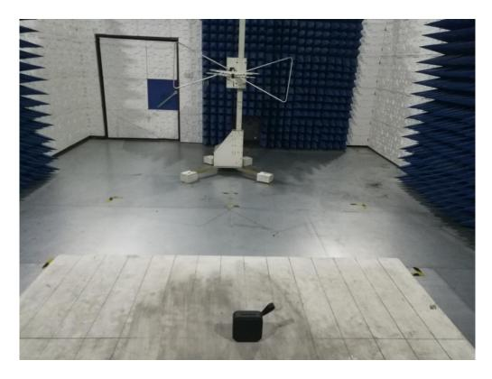
RADIATED EMISSION TEST SETUP ABOVE 1GHZ
