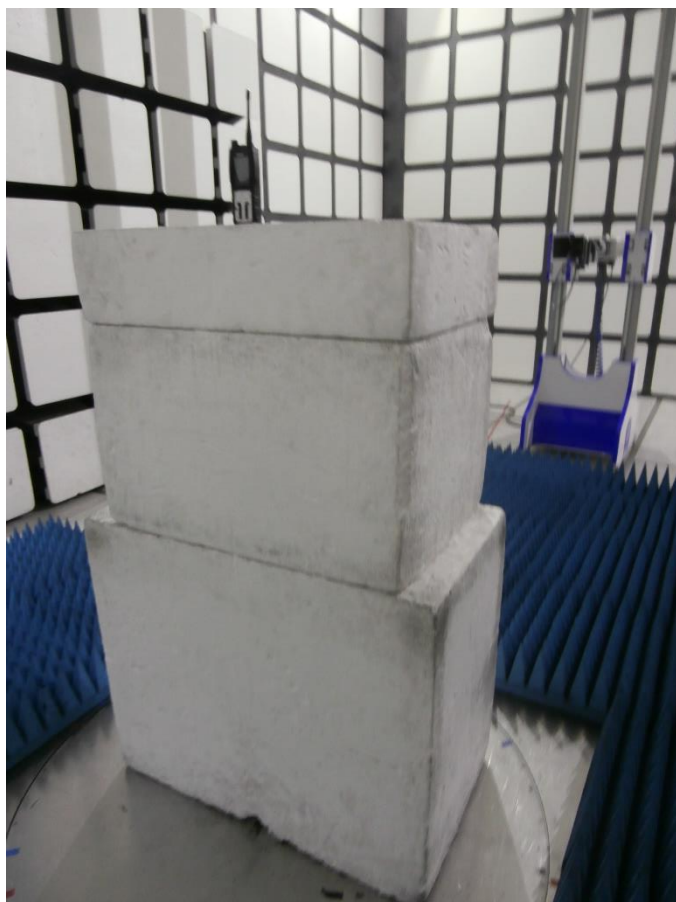
Figure 99 – Radiated Emission Setup, EUT Orientation Z
