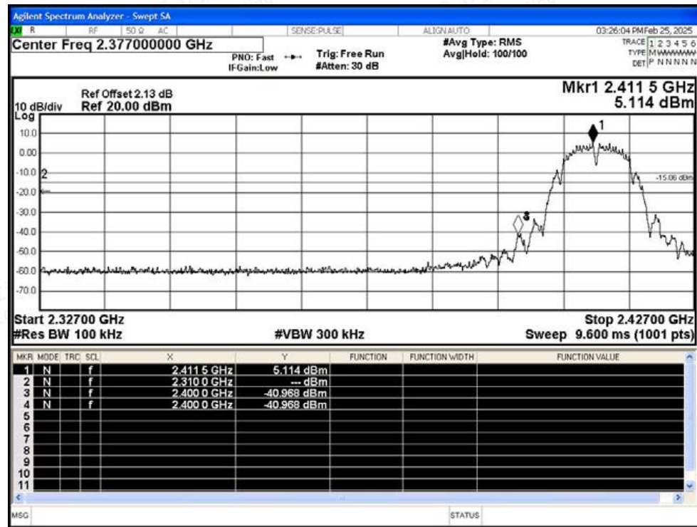
Band Edge NVNT b 2412MHz Ant1 Emission
