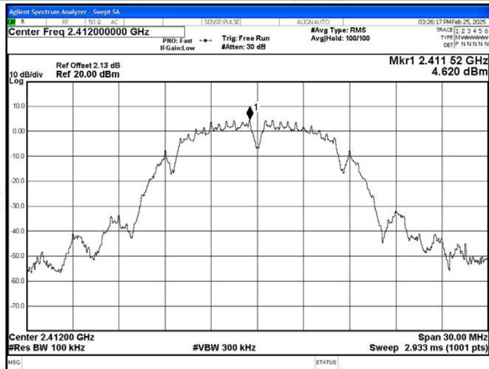
Tx. Spurious NVNT b 2412MHz Ant1 Emission
