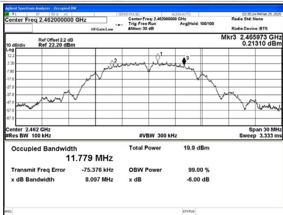
-6dB Bandwidth NVNT g 2412MHz Ant1
