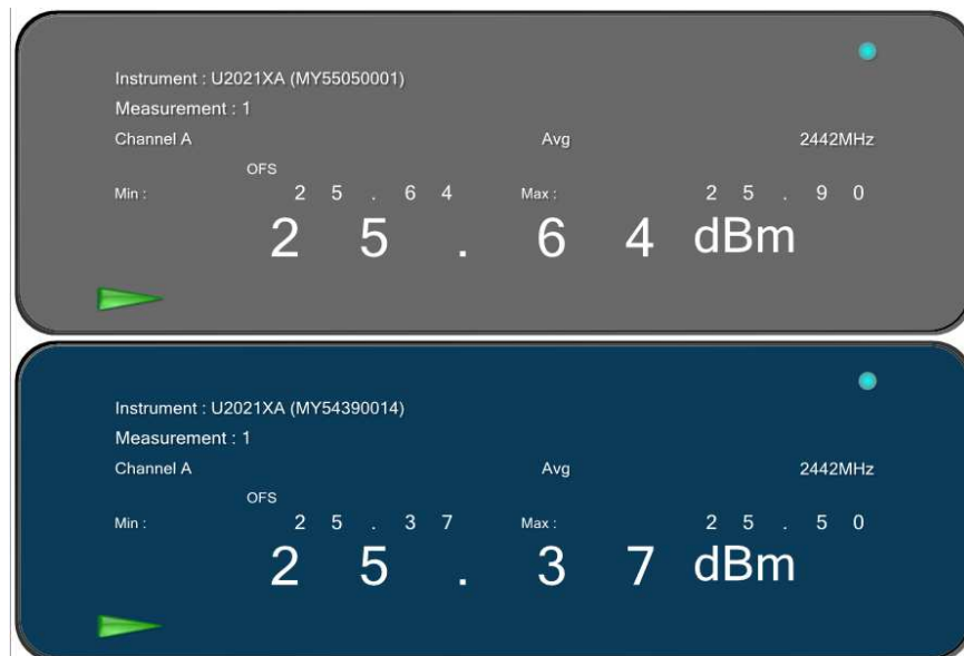
Figure 29: Maximum Conducted Output power measured at Ch.0 & Ch.1
