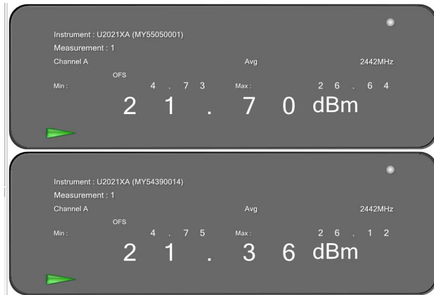
Figure 38: Maximum Conducted Output power measured at Ch.0 & Ch.1
