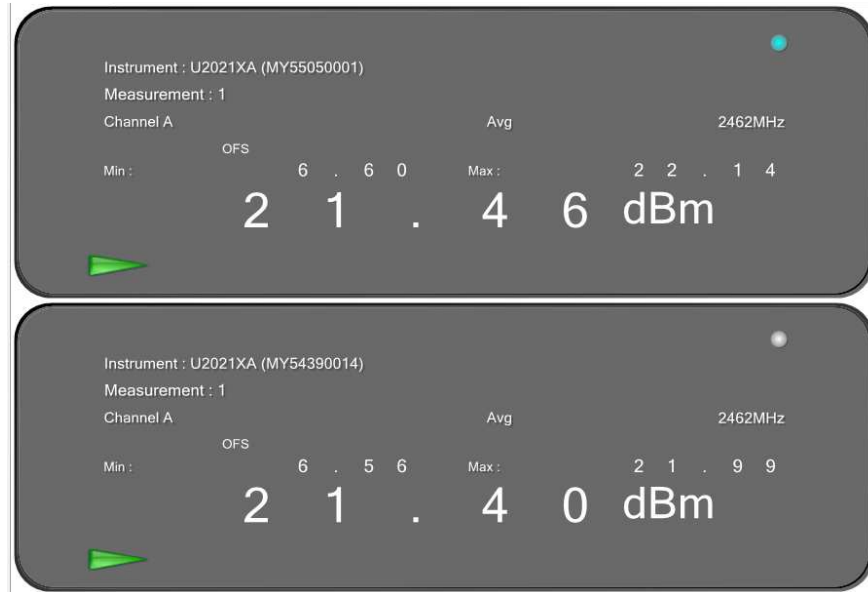
Figure 36: Maximum Conducted Output power measured at Ch.0 & Ch.1
