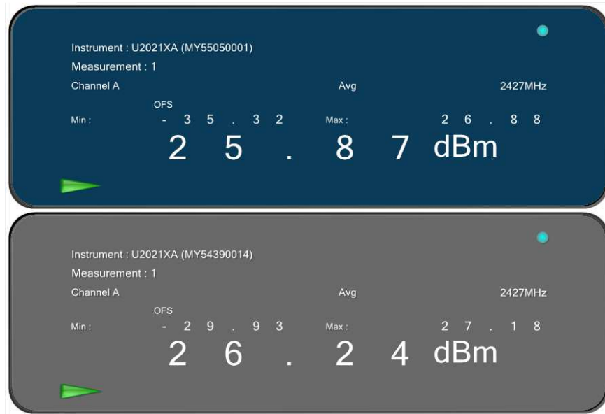
Figure 28: Maximum Conducted Output power measured at Ch.0 & Ch.1
