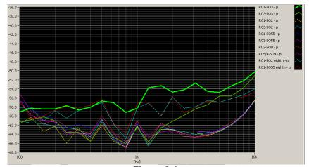
Figure 8-1 **CDMA Audio Band Magnetic Noise**
