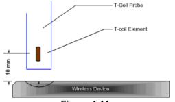
Figure 4-11 Measurement Distance
