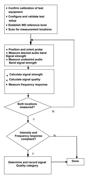
Figure 4-15 C63.19 T-Coil Signal Test Process
