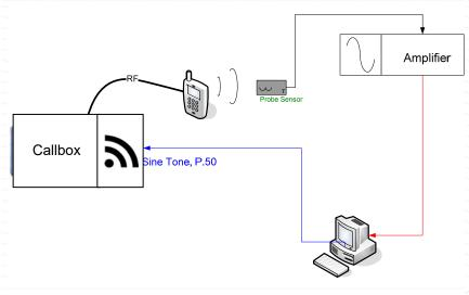
Figure 4-2 T-Coil Test Setup
