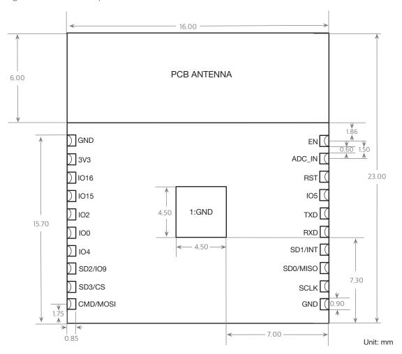
Figure 2-1. Top View of The ESP-WROOM-S2
