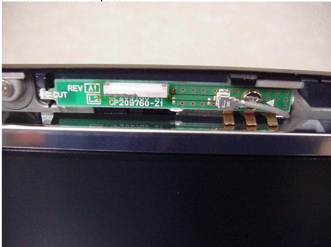
BT Antenna Location - exploded view
