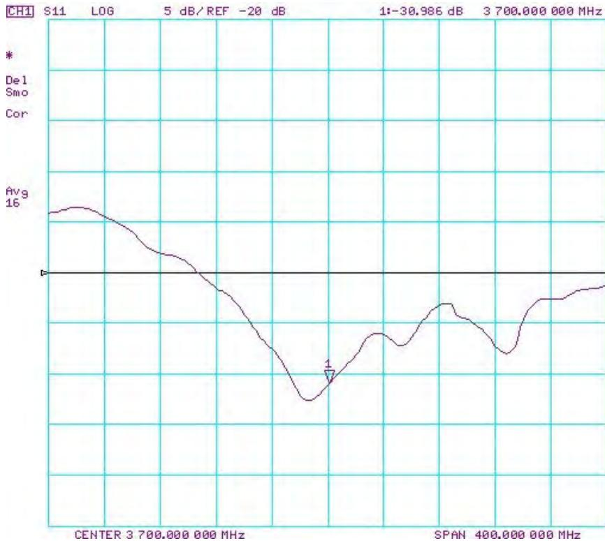
Impedance & Return-Loss Measurement Plot for Body TSL
