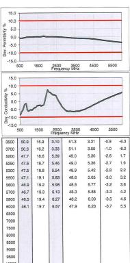
Figure D-2 600 - 6000 MHz Body Tissue Equivalent Matter
