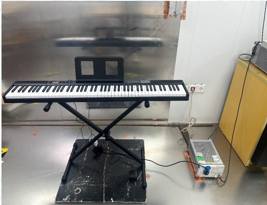
Photo of Setup for Radiated Emission (30MHz~1GHz)
