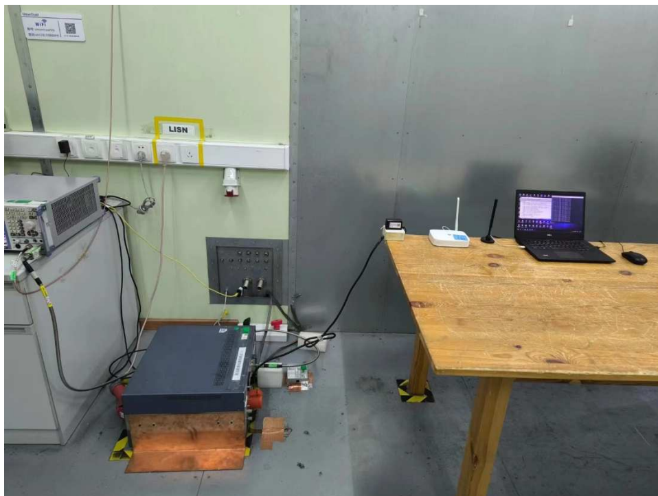
Photograph 1: Set-up for Conducted Emissions, AC Mains
