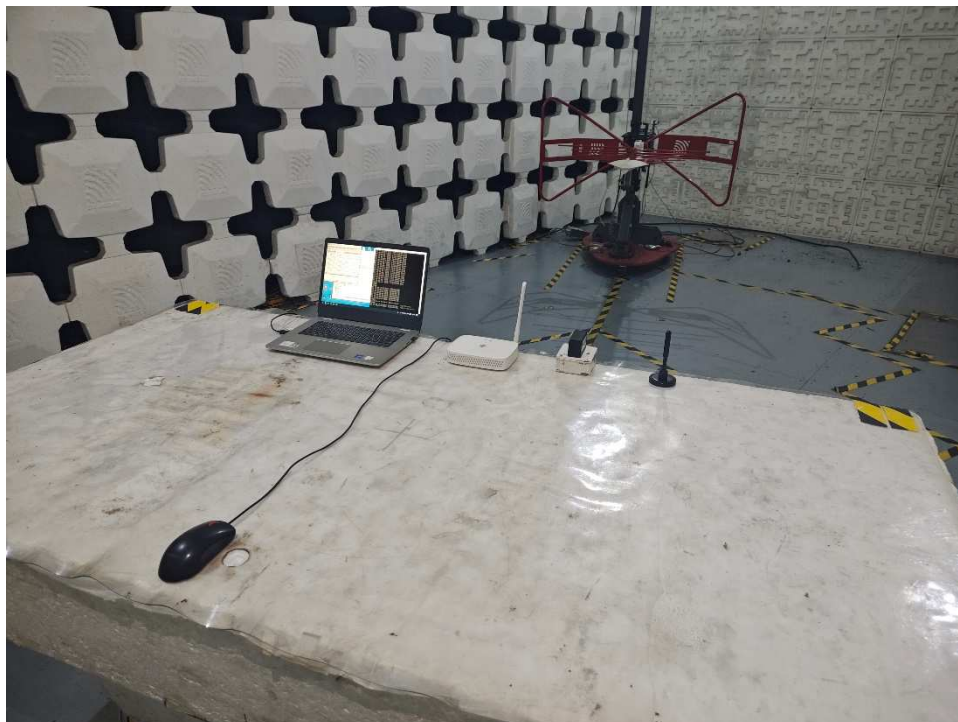
Photograph 2: Set-up for Radiated Emissions, below 1GHz
