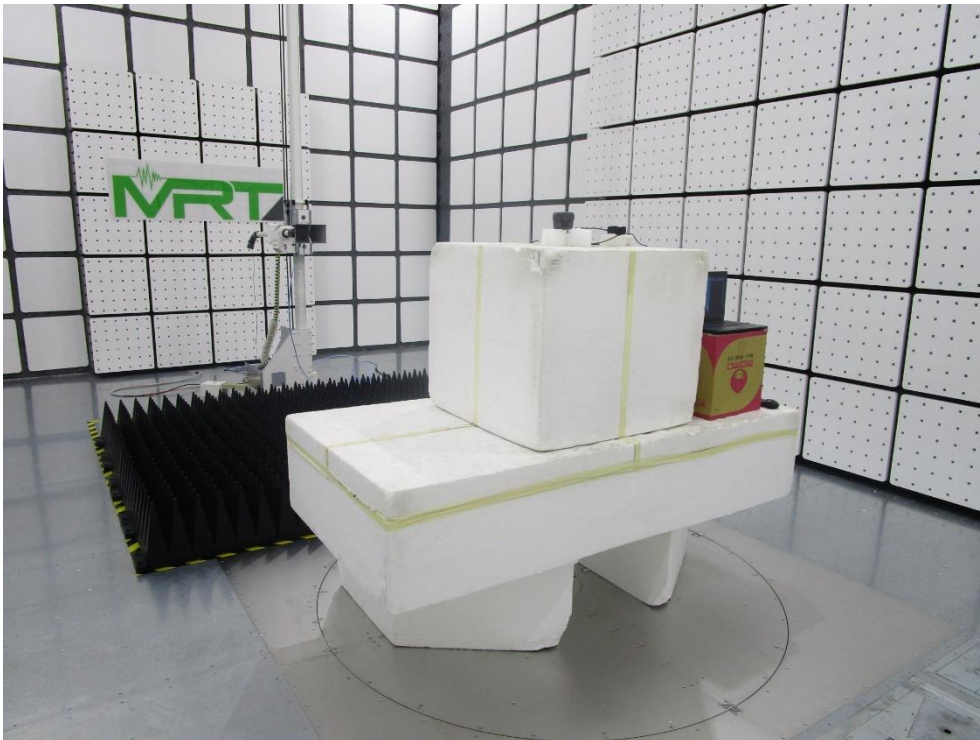
Description: Radiated Emission Test Setup for 1GHz~18GHz
