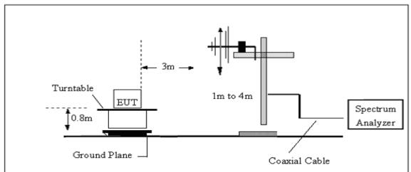
3. Radiated Emission Test-Up Frequency Above 1GHz
