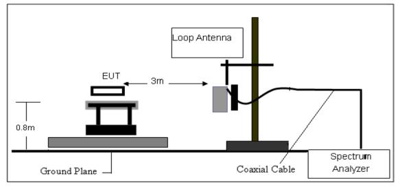
2. Radiated Emission Test-Up Frequency 30MHz~1GHz
