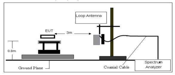
(B) Radiated Emission Test-Up Frequency 30MHz~1GHz
