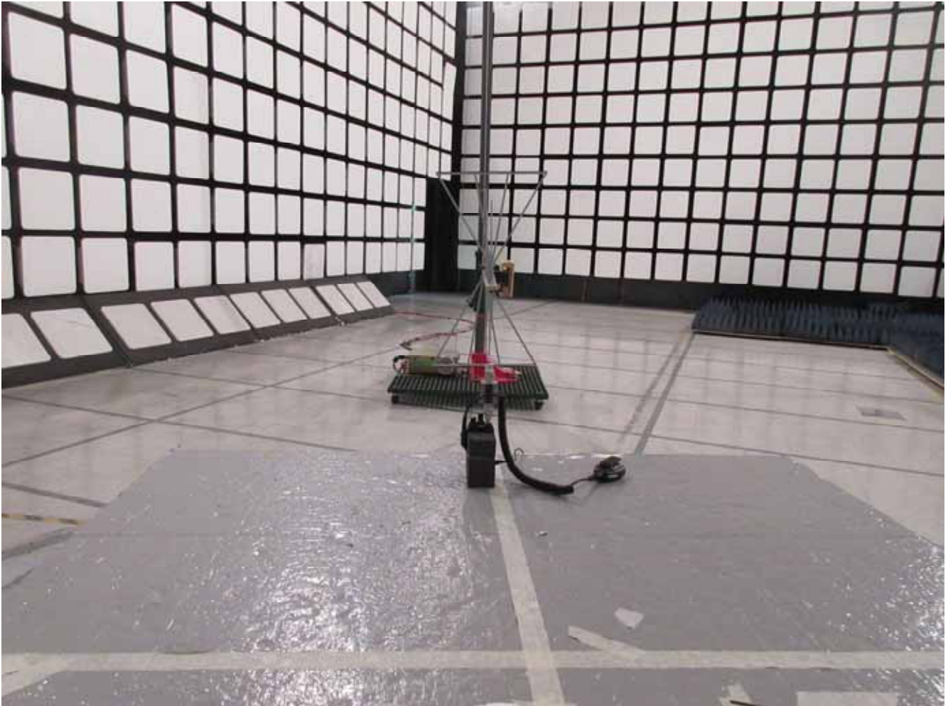
Tx Radiated Emission Test Setup
