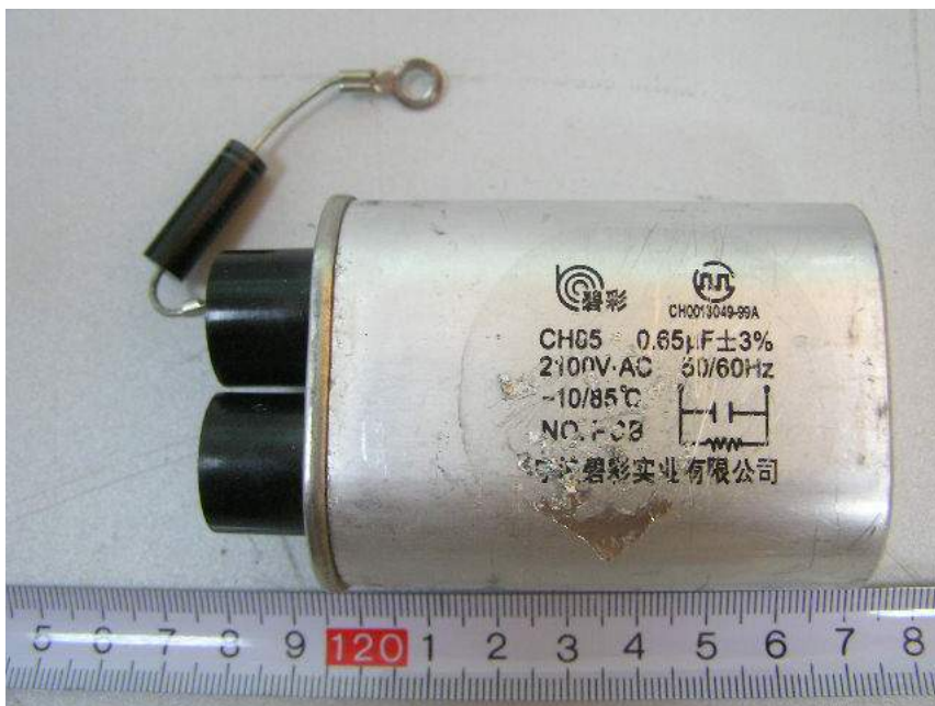
EUT – Capacitor View
