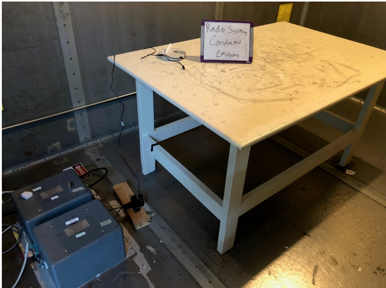
Figure 7. Powerline Conducted Emissions Test Configuration
