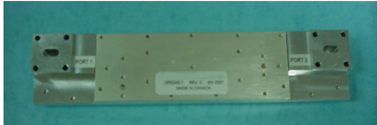
Link CX 24GHz duplexer, bottom view
