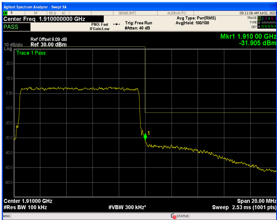
Band2 QPSK BW=15MHz Channel=18675 RB Size=1 Position=#Max
