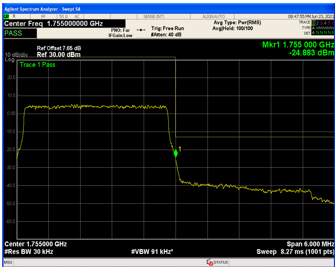
Band4 QAM16 BW=3MHz Channel=20385 RB Size=1 Position=#0
