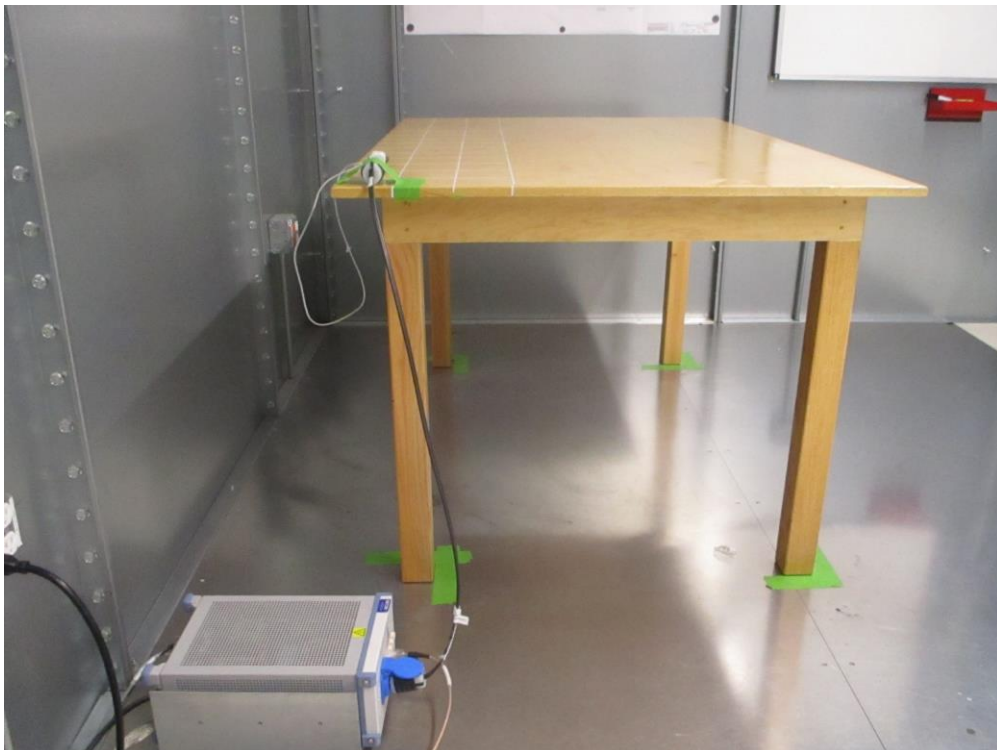
Figure 2: AC Line Conducted Emissions (Rear View)
