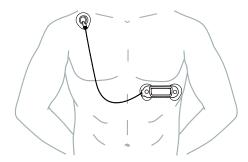
7. Once the ECG sensor is properly positioned on your body, wait half a minute then check the Q-ecg app to see if a real-time ECG reading is shown on the main screen on the app. If a real-time ECG is shown on the app, the ECG sensor has been properly worn.
