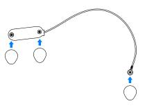
Attach the ECG sensor to the front of the sensor holder so that all four holder connectors on the sensor are properly clicked into the four sensor connectors on the holder (see image below).
