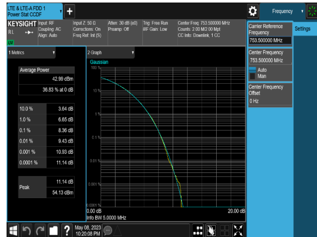
Plot 8-270. Peak To Average Power Ratio Plot (LTE B13_1C_5M_16QAM - High Channel_4T, Port 1)
