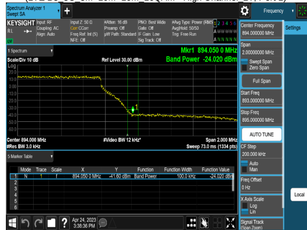
Plot 8-286. Band Edge Emission Summary Data Plot (LTE B5 2NC 5M+5M QPSK - High Channel 2T, Port 1)
