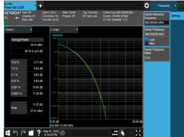
Plot 8-262. Peak To Average Power Ratio Plot (MSR 2C_DSS B(n)5_1C_10M+NR n5_1C_5M_16QAM - High Channel_4T, Port 0)
