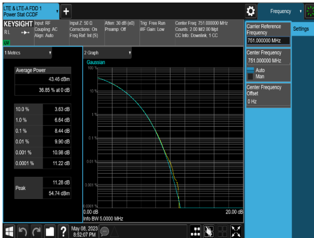
Plot 8-269. Peak To Average Power Ratio Plot (LTE B13_1C_5M_QPSK - Mid Channel_4T, Port 0)
