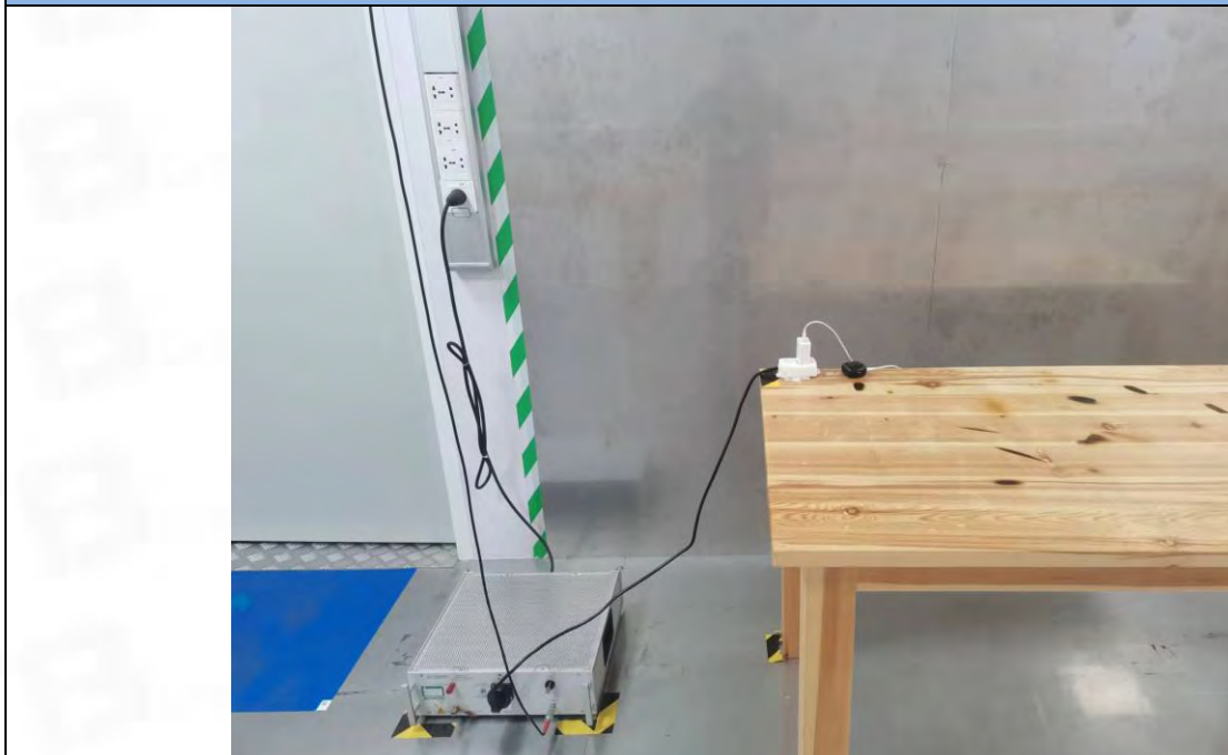
Conducted Emission at AC power line
