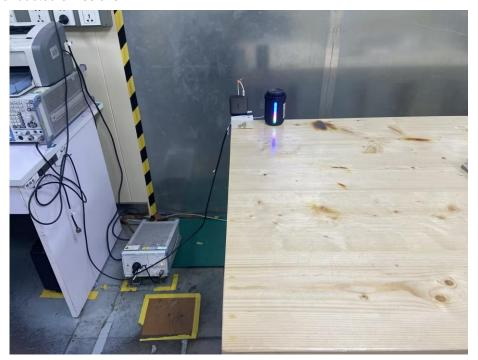
Spurious Emission Test Setup (Below 1GHz)
