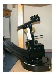
Larger DUT's (e.g. notebooks) cannot be tested using this device holder. Instead a support of bigger polystyrene cubes and thin polystyrene plates is used to position the DUT in all relevant positions to find and measure spots with maximum SAR values.
