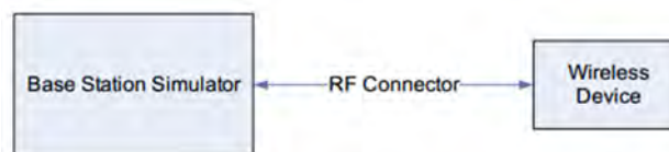
Figure 9.1 Power Measurement Setup
