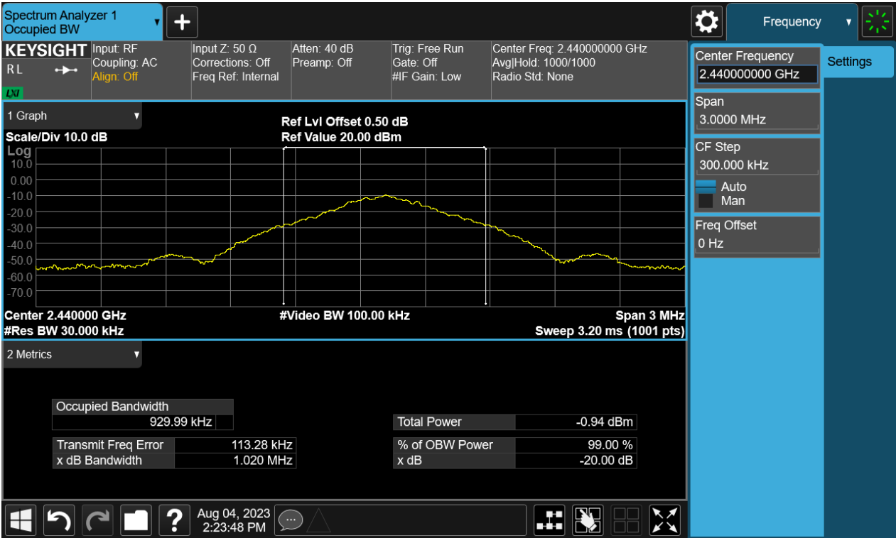
Figure 30: The plots of 20dB Bandwidth and 99% Bandwidth, 2440MHz
