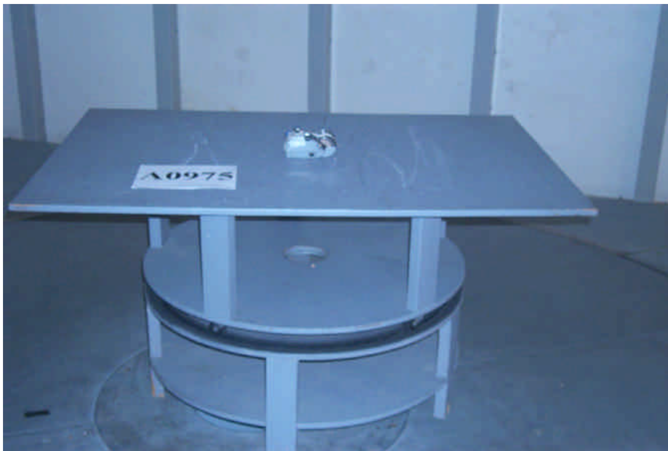
Radiated Emissions Side 1 on the Cameo 3 printer
