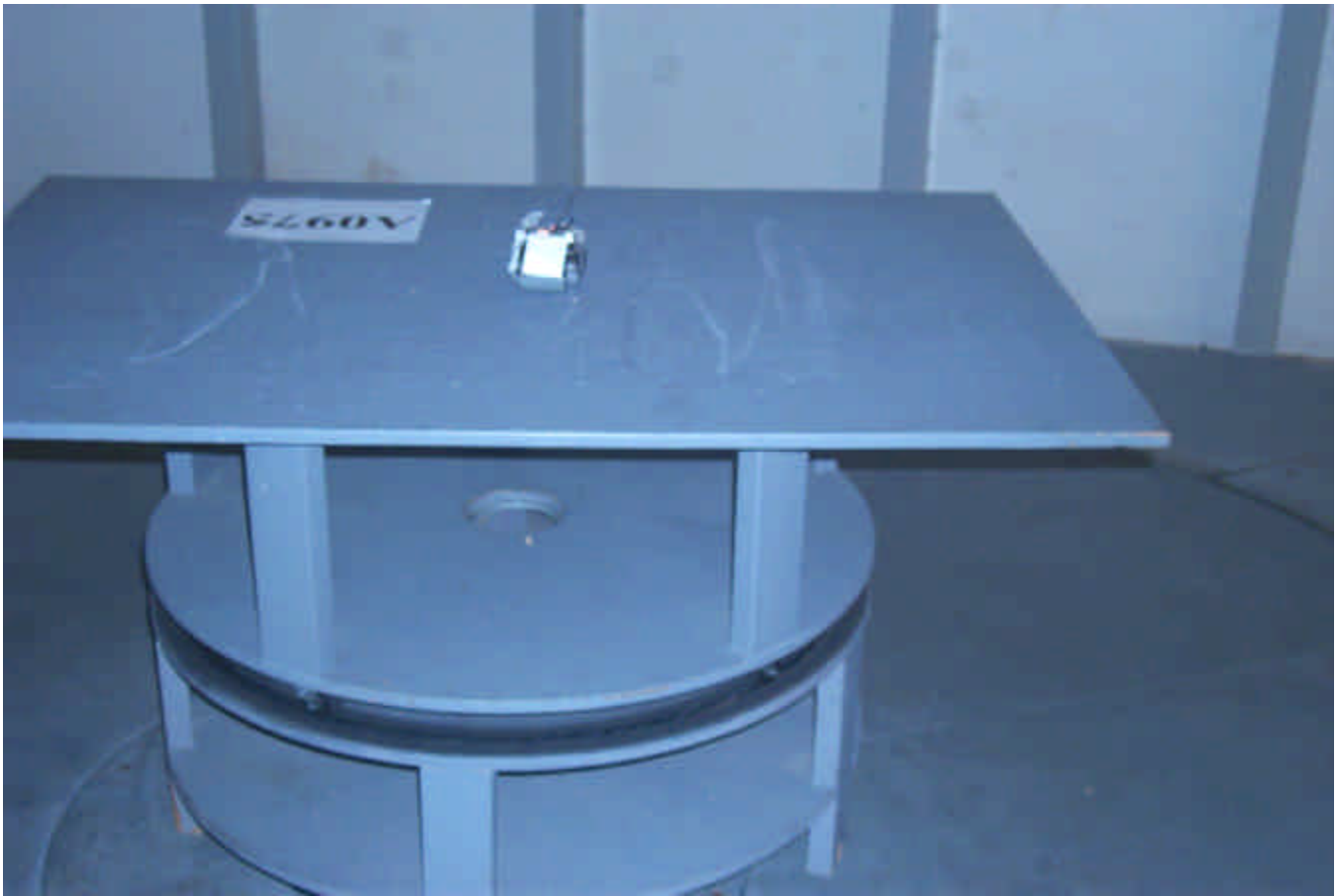
Radiated Emissions Side 2 on the Cameo 2 printer
