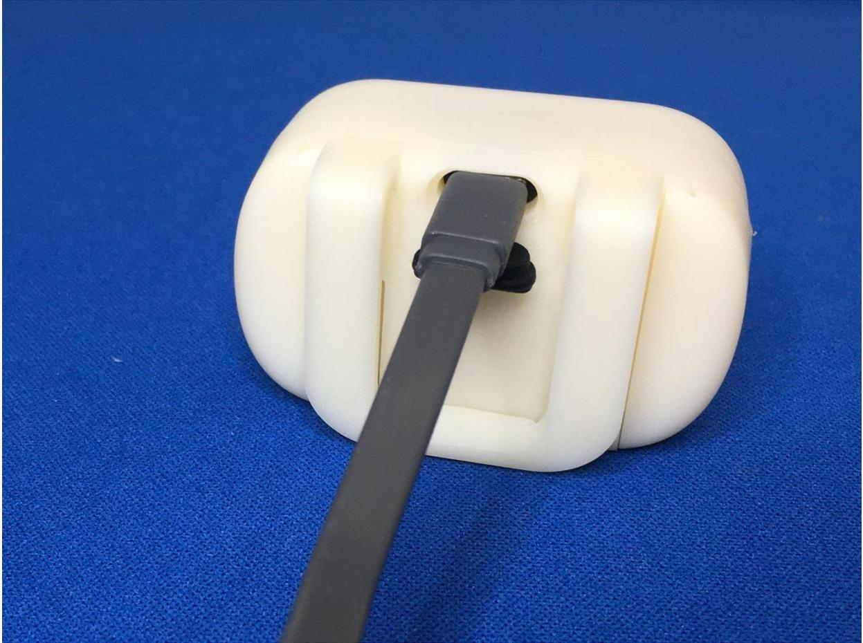
*Figure 3 Link 3 - Back showing cable inserted in charging port through clip.*
