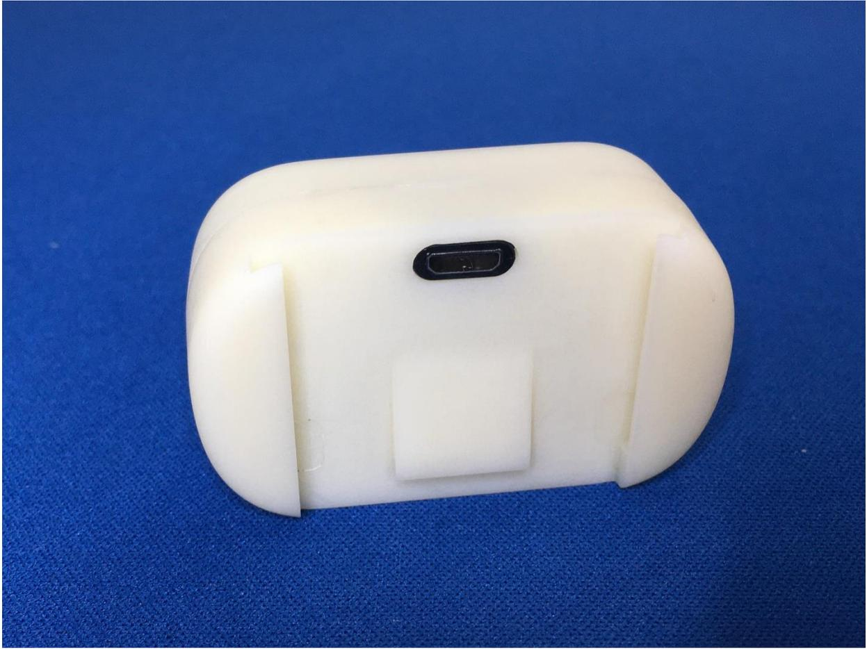
*Figure 2 Link 3 - Back showing charging port without clip.*
