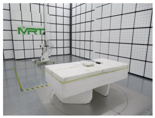
Description: Radiated Spurious Emission Test Setup for above 1GHz (2.4G Wi-Fi & 5G Wi-Fi Band 3, 4)
