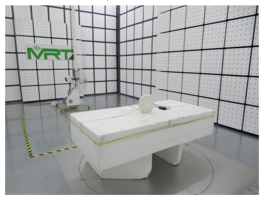
Description: Radiated Spurious Emission Test Setup for above 1GHz (BLE & Scan Antenna & 5G Wi-Fi Band1, 2)
