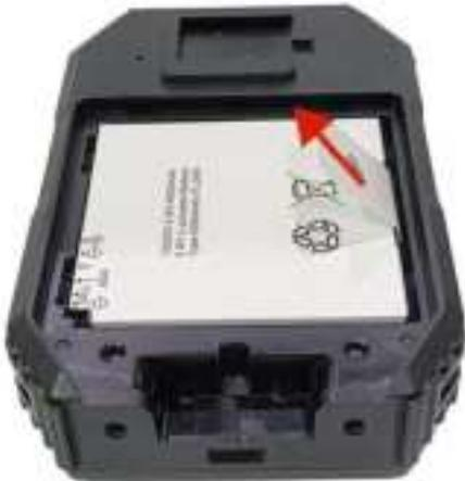
Step 3. Use the screwdriver or pen to press on the reset button or press and hold on the button for resetting (Resetting can only achieve the BWC hardware reset, modifying relevant parameters is not supported).
