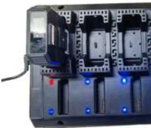
Step 4. After BWC inserting the station or Dock, BWC will automatically obtain the IP address assigned by the router (DHCP mode). After successful acquisition, it will display the IP on the LCD screen (as shown in the figure below) for 5 seconds.
