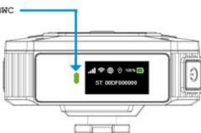
Step 4: Insert the battery into the dock. The battery light of the dock turns red or green. (If the battery is not fully charged yet, the battery light is red. If the battery is fully charged, the battery light is green.) The following figure shows that the battery is fully charged and the battery light is green.)
