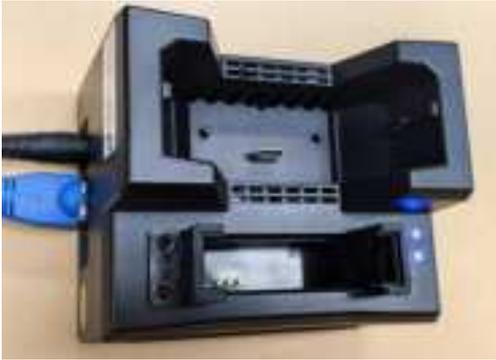
Step 2. Insert the BWC vertically into the dock. The dock status light turns red, and the dock is successfully connected to the BWC (see the following figure).
