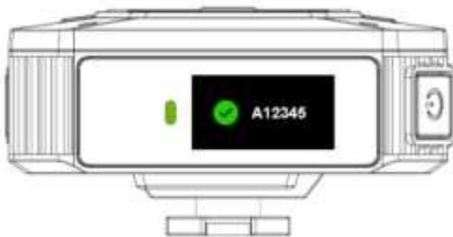
Step 3. The standby status is restored and displayed on the LCD of the BWC after 5 seconds.
