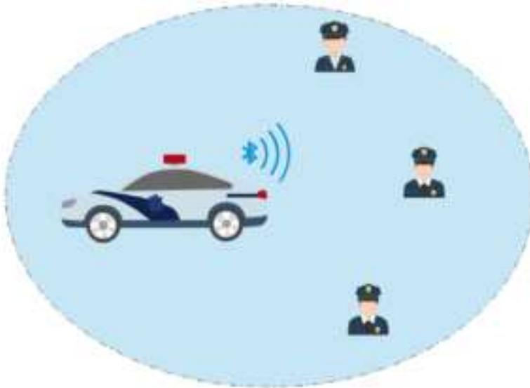
Step 2. The MDVR activates recording on the BWCs paired with it in the signal coverage (about 10 meters) , and the recording icon overlapped with the Bluetooth linkage icon is displayed on the LCD (see the following figure).
