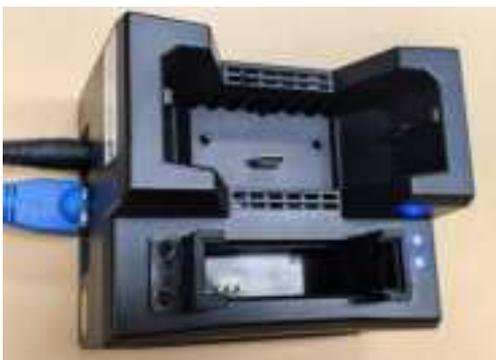
Step 2. Insert the BWC vertically into the dock (see the following figure). The dock status light turns
