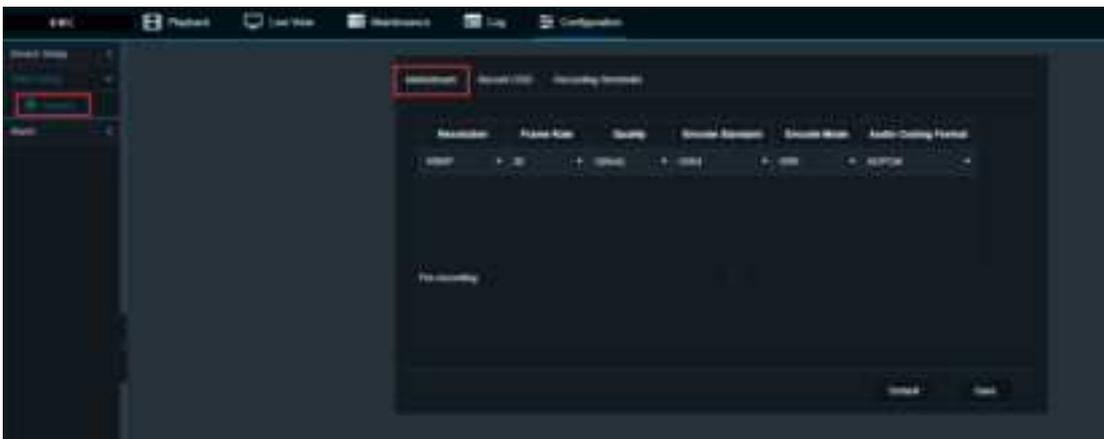
You can set resolution, frame rate, picture quality, encoding format, encoding mode, audio mode.
