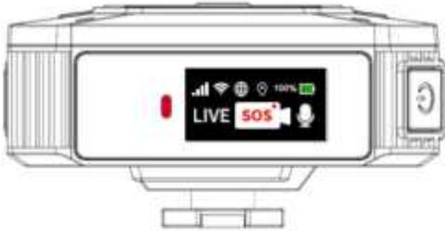
Step 4. A "LIVE" icon is displayed on the left side of the LCD, as shown in the following figure. This icon will be displayed until the platform monitoring or BWC recording is stopped.
