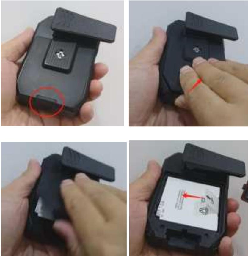
Note: When take out the battery, you need to pull the sticker to the left side, but not upwards.
