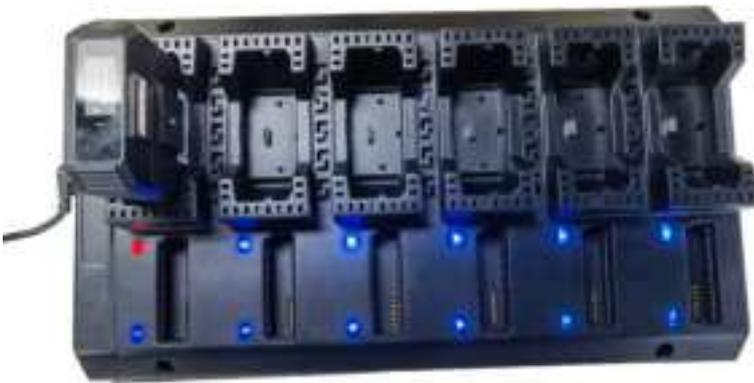
Step 3. Insert the battery into the Station. The battery light of the Station turns red or green. (If the battery is not fully charged yet, the battery light is red. If the battery is fully charged, the battery light is green. The following figure shows that the battery is fully charged and the battery light is green.)
