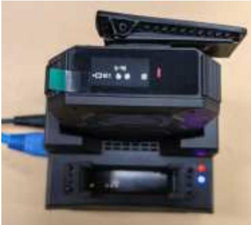
Step 3. If there is video evidence in the BWC needing to be uploaded and synchronized to the platform, the dock can upload the data automatically, and the status bar and upload progress are displayed on the LCD (see the following figure).
