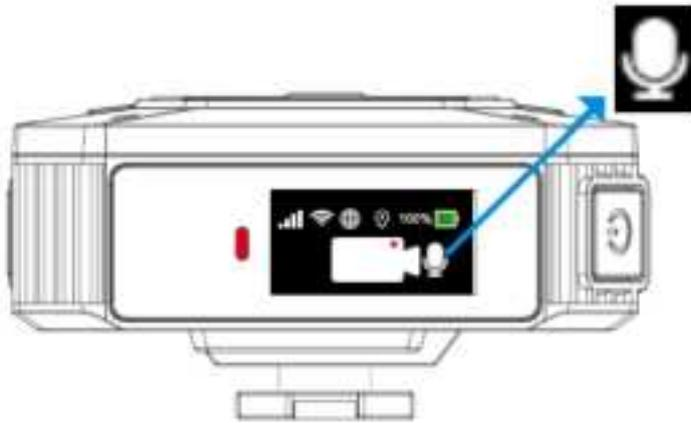
Step 2. Double-press the FN button on the side of the BWC.
