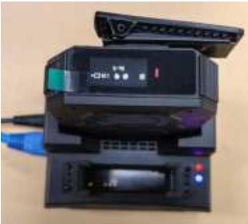
Step 3. When a BWC is not fully charged yet, the status light on BWC is blinking. After the BWC is fully charged, the status light on BWC turns solid.
