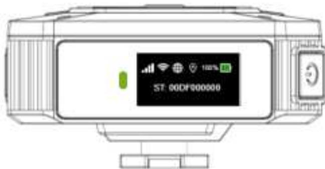
Step 3. In the standby mode, the BWC status and policeman ID are displayed on the LCD (if the BWC is powered on for the first time, no policeman ID is displayed until the ID is configured). On the upper part of the LCD, the status icons for the 4G signal, AP hot spot status, server (platform) connection status, GPS positioning, battery percentage, and battery level are displayed in turn.
