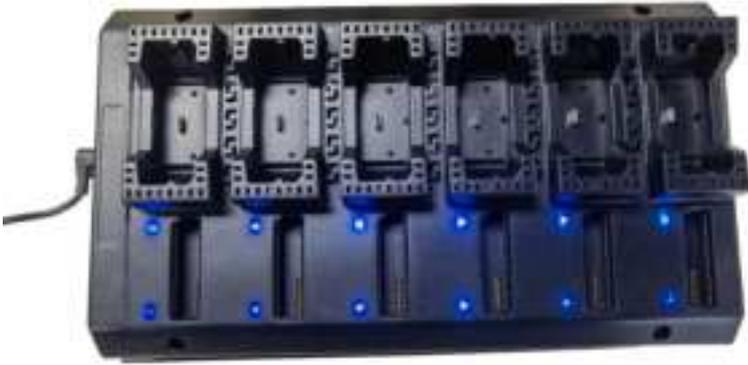
Step 2. Insert the BWC vertically into the Station. The BWC light on the Station turns red, indicating the connection is successful (the light indications are the same as the dock).
