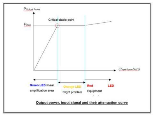
P<sub>Output Power</sub>: Output Power P<sub>input Power</sub>: Input Power V<sub>ATT</sub>: Attenuation value of attenuator P<sub>input Power</sub> -V<sub>ATT</sub>: Input Power—Attenuation value of attenuator P<sub>max</sub>: Rate output power
