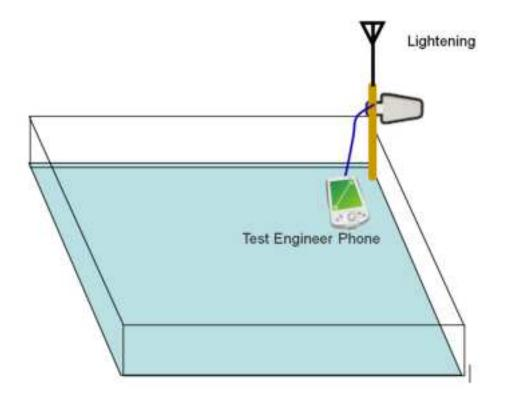
Fix the donor antenna after selecting the best position, and adjust slightly its height or angles in order to get the signals with suitable input power level and calling quality.
