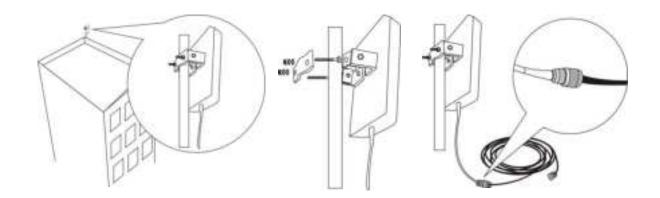
Installation of wide directional antenna as donor antenna
