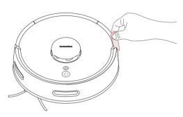
3. Remove the faceplate and flip the ON/OFF switch to "I".
