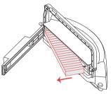
Remove the debris by tapping the filter against your trash container.
