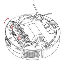
2. Remove the brush from the robot by holding its left end. Remove the brush caps from the end. Use the small cleaning tool to remove any hair and debris that has collected beneath the caps. Reinstall the brush cap.
