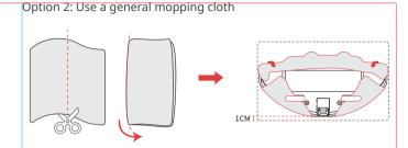
Please note: Dimensions of a general mopping cloth is usually approx.  $30 \times 20$  cm (11.8 × 7.9 in.), while your robot's mopping pad plate is compatible with 20 × 15 cm (7.9 × 5.9 in.) cloth. If you use a general mopping cloth, fold or cut it in half before attaching to the mopping pad plate.
