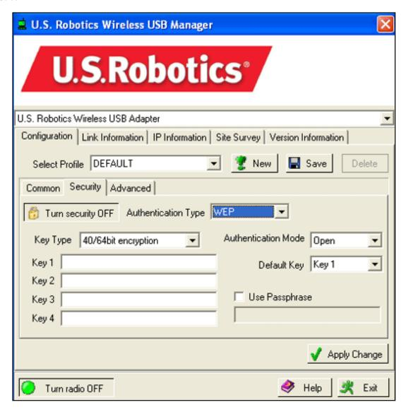
WEP is an encryption scheme that is used to protect your wireless data communications. WEP uses a combination of 40/64-bit keys or 104/128-bit keys to provide access control to your network and encryption security for every data transmission. To decode a data transmission, each wireless client on the network must use an identical 64-bit or 128-bit.
