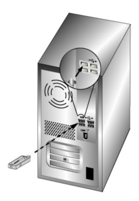
**Note:** Make sure the 802.11g 54Mbps USB Adapter is fully inserted into the USB port on your computer so that the 802.11g 54Mbps USB Adapter is detected.
