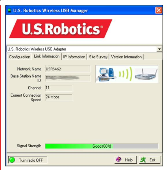
You will see a picture with a computer and a wireless device. If you see a graphic representing signal waves between the computer and the wireless device, you are connected to the wireless network.
