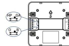
9. Gently push the thermostat down onto the back plate. You may hear an audible click, as it snaps into place. Observe the rear thermostat sides, near the wall, to ensure there are no uneven gaps between the plate and the thermostat. Gently tug on the thermostat, to ensure it does not come loose.
