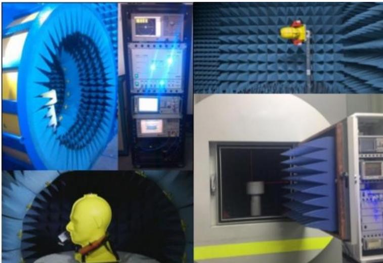
Our company has a number of OTA test darkrooms, ranging from 400MHz to 8.5ghz, which can provide passive test and active test (including OTA overall 2G,3G,4G,5GFR test, WiFi multi-mode test, GPS active test, Bluetooth active test, which can provide antenna gain and efficiency. 2D orientation and apple chart analysis and upper and lower hemisphere efficiency values, mutual disturbance correlation coefficient test items
