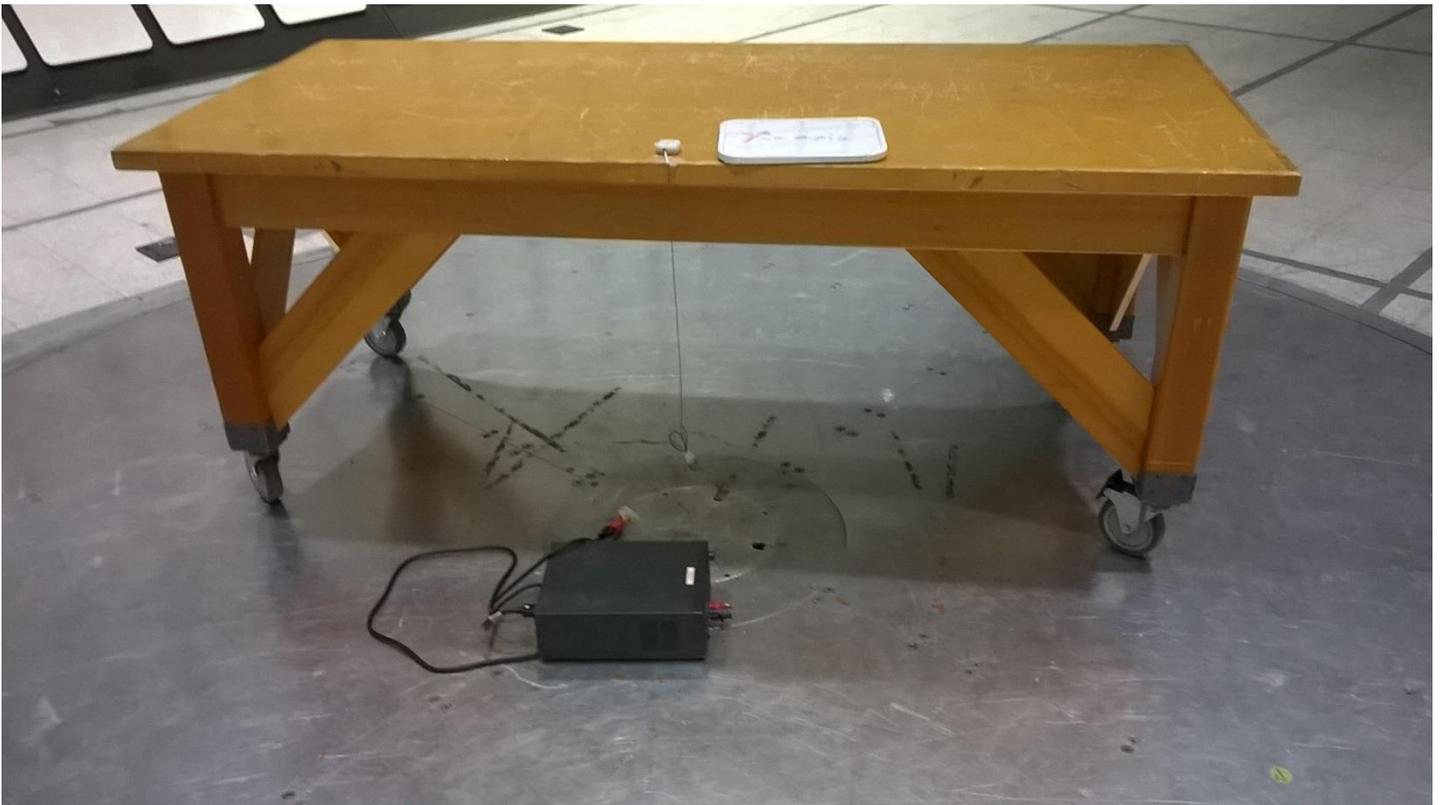
**Figure 1 – Radiated Emissions Test Setup, 30MHz – 1GHz**
