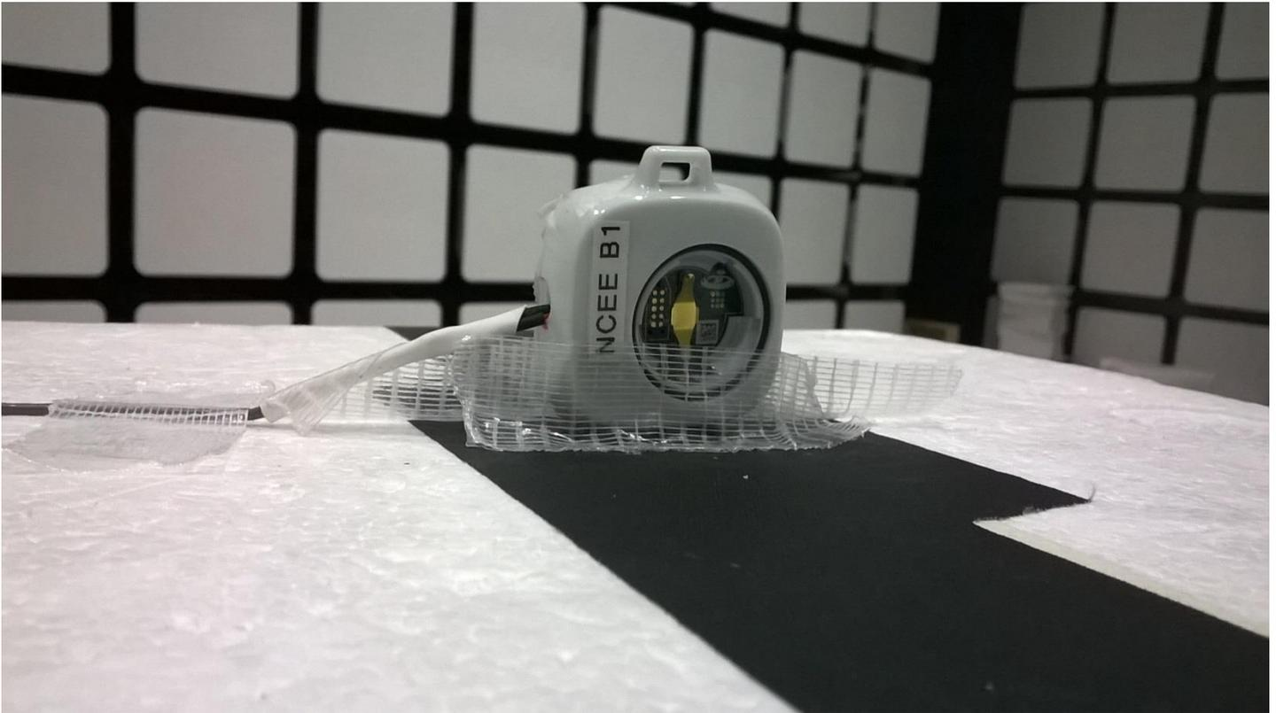
Figure 2 - Radiated Emissions Test Setup, 1 – 19 GHz
