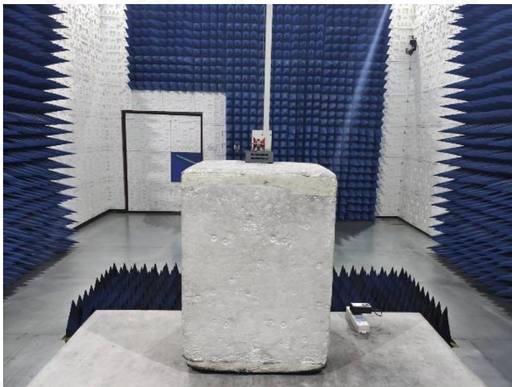
FCC RADIATED EMISSION TEST SETUP ABOVE 1GHZ
