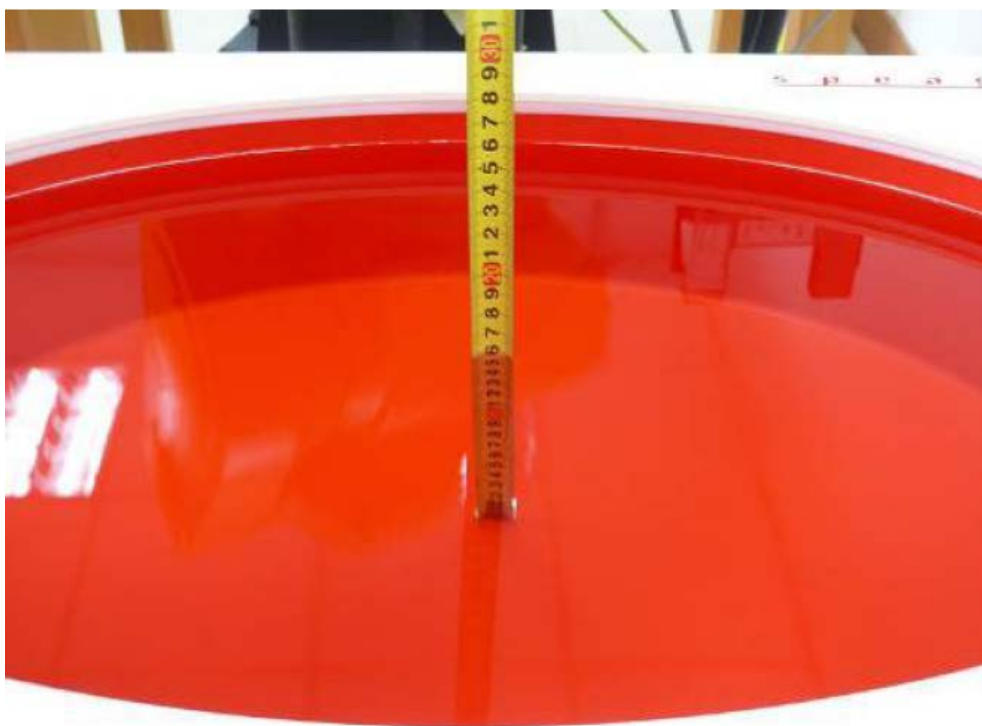
Photograph of the depth in the Body Phantom (15.3cm depth)
